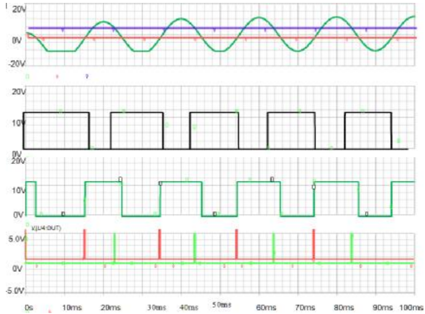
Figure (5) O/p of firing circuit stages.
