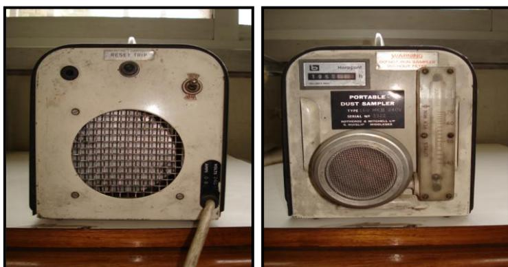
**Figure 2-** Front and back view of Low Air Sampler (Sniffer) devise features.
