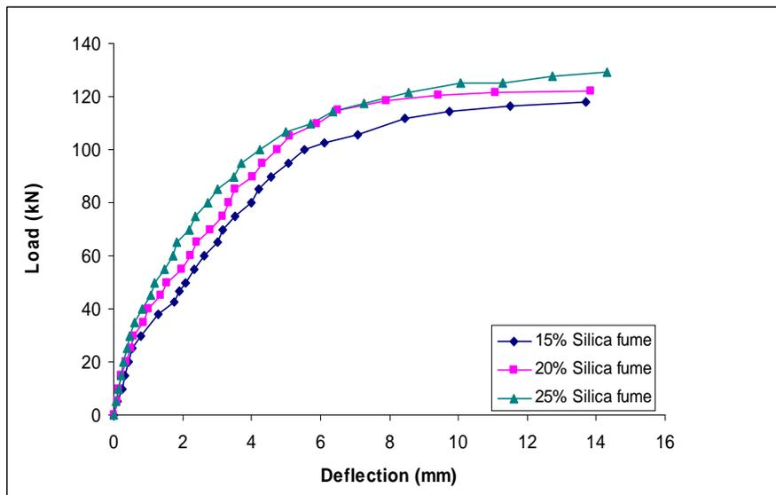
Fig .(7) Effect silica fume ratio on load-deflection curves of RPC T-beams
