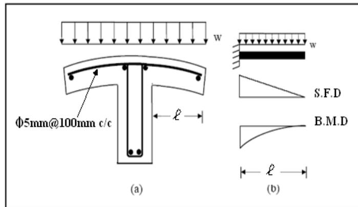
Fig .(2) (a) Transverse bending of T-beam flange (b) Shear and moment diagrams for flange overhang
