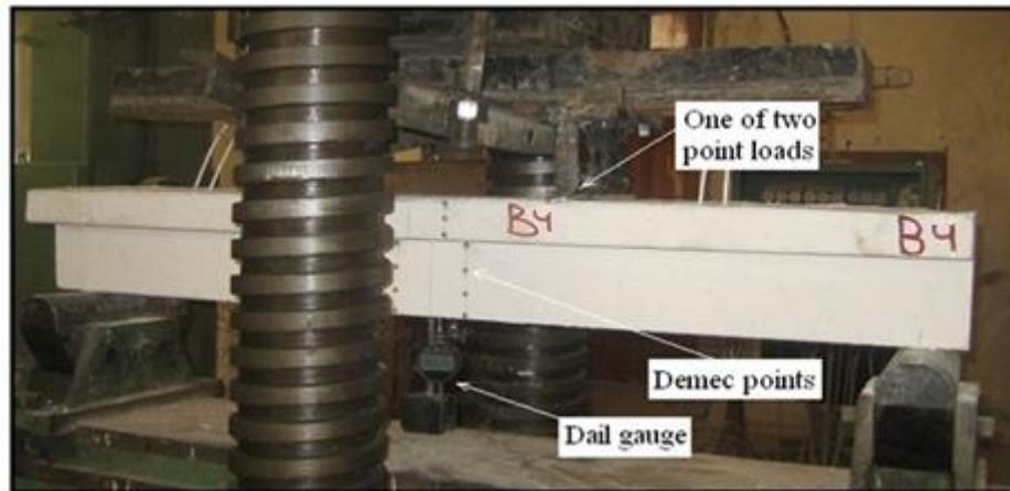
Fig .(5) One of the beams under testing
