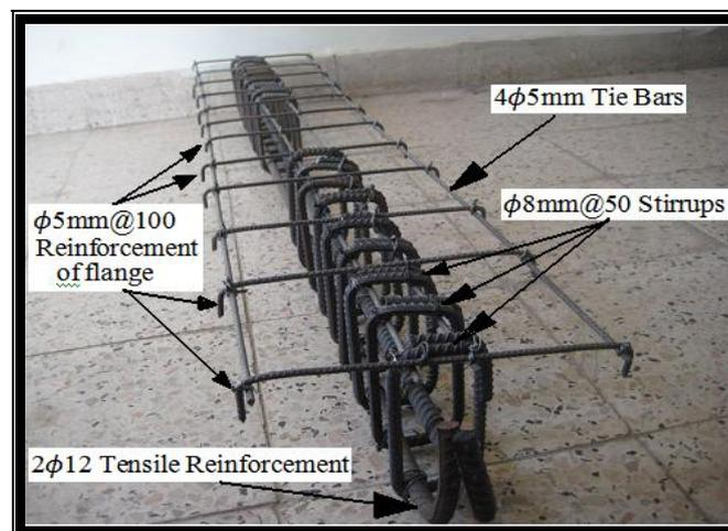
Fig .(3) Details of flexural beam reinforcement
