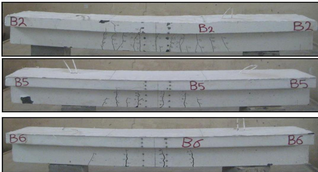
**Fig .(8) Effect steel fibers volumetric ratio on crack pattern of RPC T-beams**
