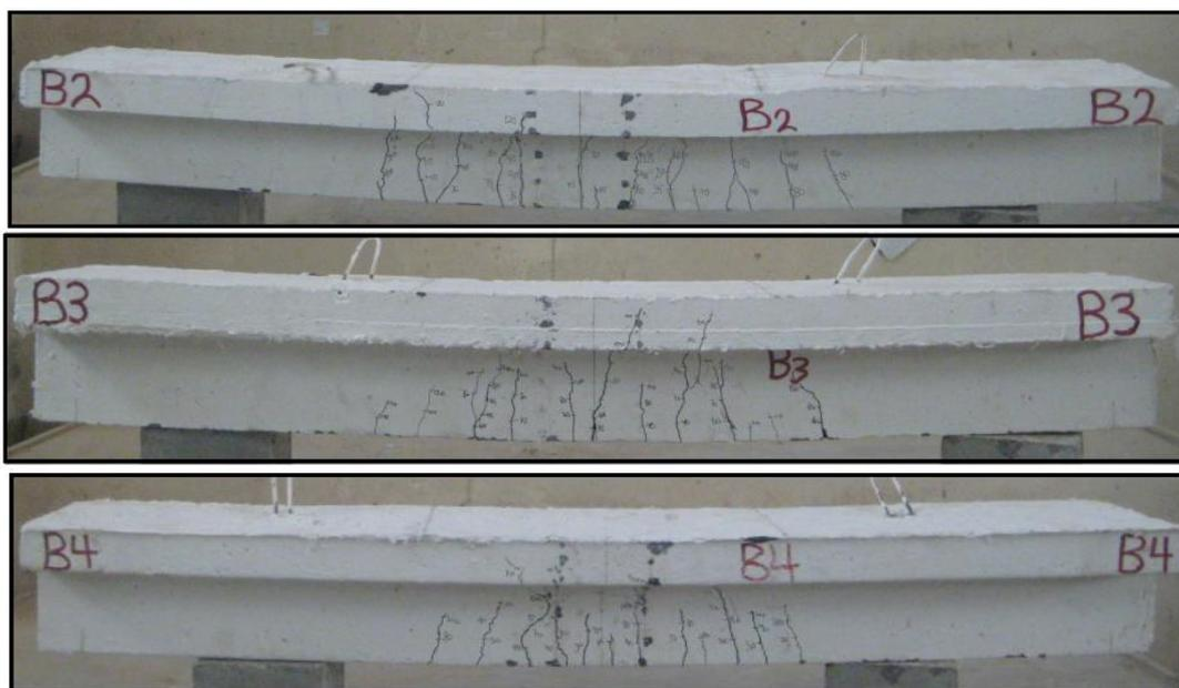
**Fig .(9) Effect silica fume ratio on crack pattern of RPC T-beams**
