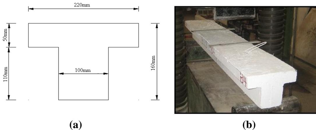
**Fig .(1) Details of tested beams (a) Beam cross-section (b) Isometric plate**
