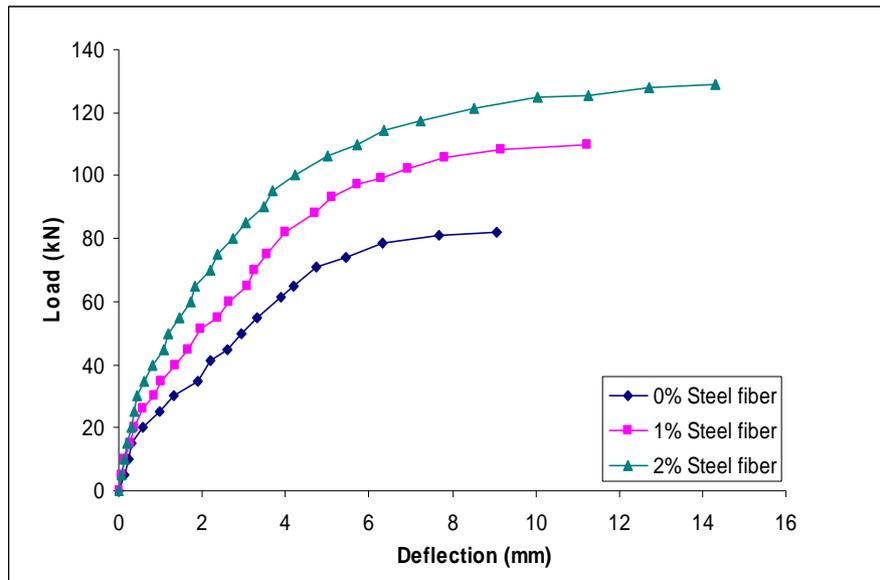
Fig .(6) Effect of steel fibers volumetric ratio on load-deflection curves of RPC T-beams
