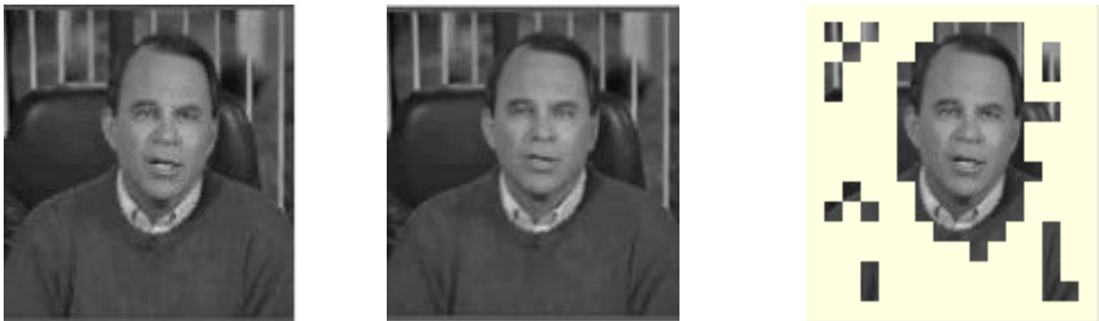
Figure 4- The Reconstruction image (I) and (P) when block truncation applied for man The number of block difference 90 if select thr. 4 using MAD
