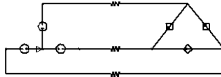
(a) Thevenin equivalent circuit for the three phase supply network connected to the delta connected stranded coil circuit elements to feed the three phases of the transformer FE model.
