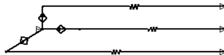
(b) Secondary load circuit represented by three stranded coil circuit elements, star connected with earthed common point, and a 3 phase resistive load.
