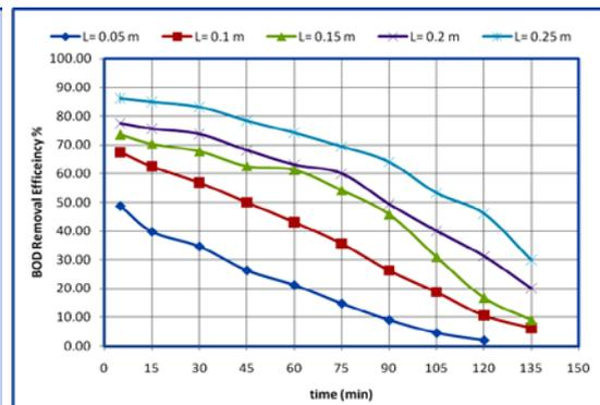
Figure (11): Adsorption removal efficiency for different packed heights.
