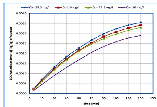
Figure (2): Adsorption rate for different BOD<sub>5</sub> influent initial concentrations.
