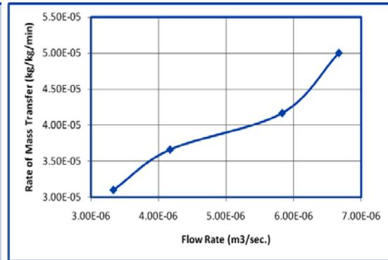
Figure (9): effect of the influent flow rates on the rate of mass transfer of BOD<sub>5</sub>.
