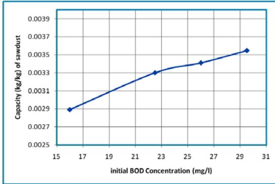
**Figure (3):** effect of the influent initial BOD<sub>5</sub> concentrations on the capacity of the sawdust.
