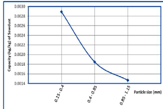
**Figure (17)** effect of particle sizes on the capacity of sawdust
