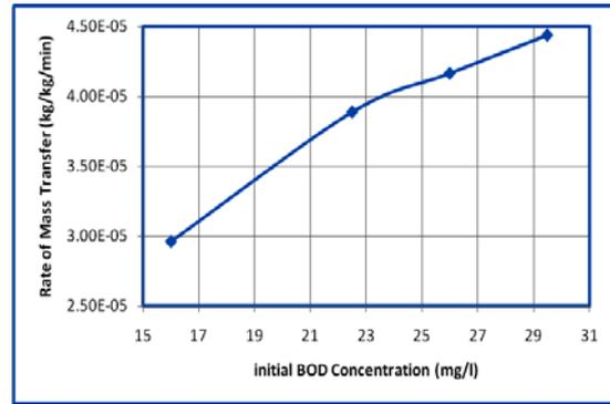
**Figure (4):** effect of the influent initial BOD<sub>5</sub> concentrations on the rate of mass transfer.
