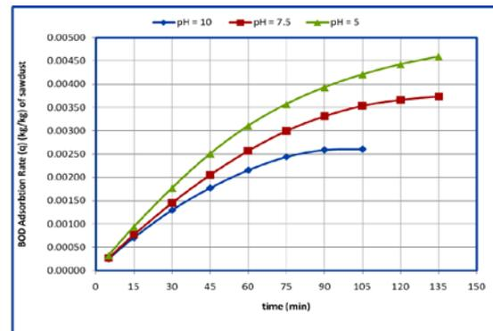
**Figure (20):** Adsorption rates of different influent pH.
