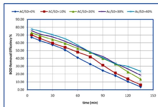
**Figure (23)** the effect of the AC/SD ratios on the BOD<sub>5</sub> removal efficiency.
