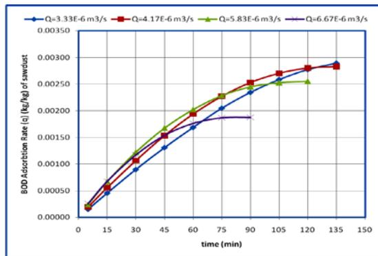
**Figure (7):** Adsorption rate for different influent flow rates.
