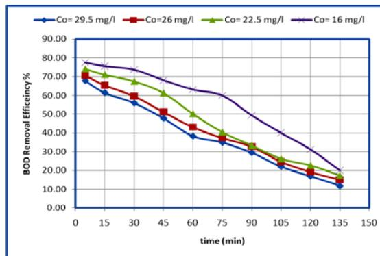
**Figure (5):** effect of the influent initial BOD<sub>5</sub> concentrations on the adsorption removal efficiency of sawdust.
