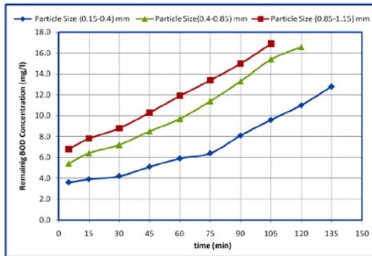
**Figure (14)** Breakthrough curves of isothermal adsorption for different particle sizes.
