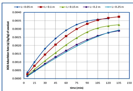
Figure (12): Adsorption rate for different packed heights.
