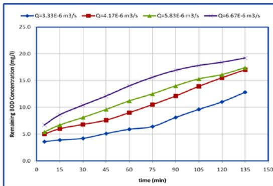
**Figure (6)** breakthrough curves of isothermal adsorption for different influent flow rates.
