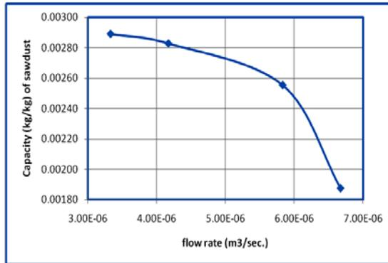
Figure (8): effect of the influent flow rates on the capacity of the sawdust.
