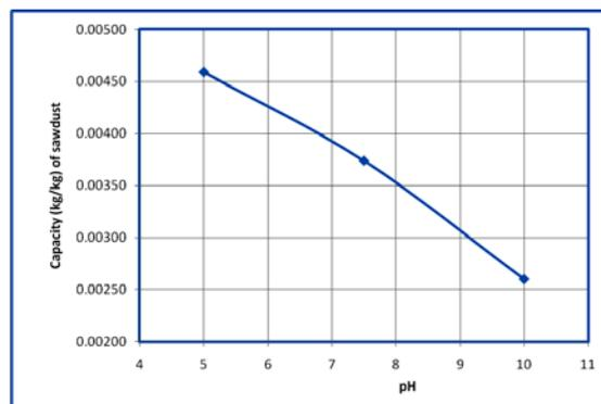
**Figure (21):** effect of the pH of the influent on the capacity of the sawdust.
