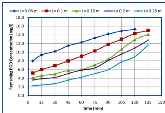
Figure (10): breakthrough curves of isothermal adsorption for different packed heights
