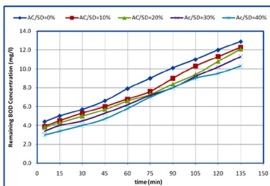
**Figure (22)** breakthrough curves of isothermal adsorption for different AC/SD ratios.
