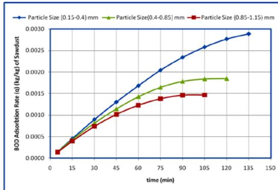
**Figure (16)** Adsorption rate for different particle sizes.
