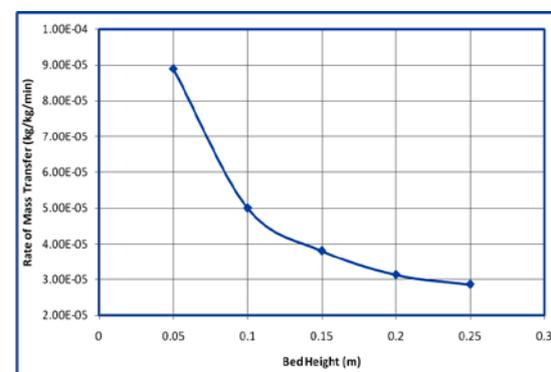
Figure (13): effect of the bed heights on the rate of mass transfer of BOD<sub>5</sub>.
