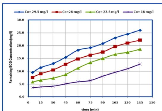
Figure (1): breakthrough curves of isothermal adsorption for different BOD<sub>5</sub> influent initial concentrations.
