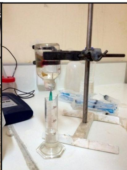
**Figure3.** Gas collection by displacement.
