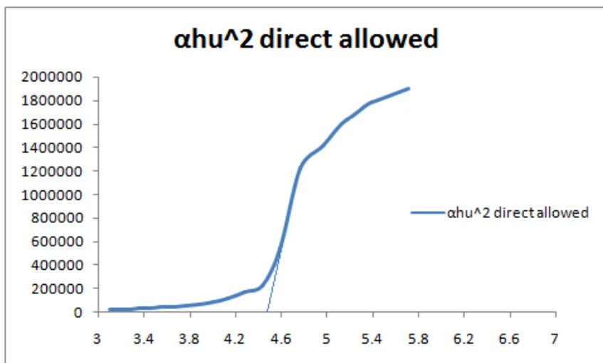
Fig. (3) Allowed direct transition  $(\alpha h\nu)^2$  Vs. Energy for the sample P2.
