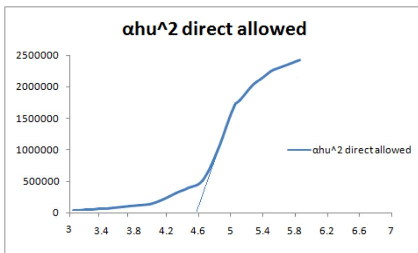
Fig. (6) Allowed direct transition  $(ahv)^2$  Vs. Energy for the sample P5.
