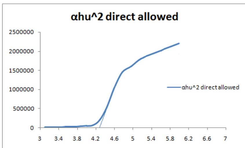
Fig. (5) Allowed direct transition  $(\alpha h\nu)^2$  Vs. Energy for the sample P4.
