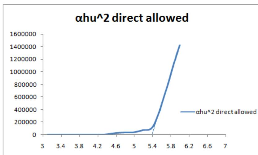
**Fig.(1) Allowed direct transition  $(ah\nu)^2$  Vs Energy for pure PVC.**
