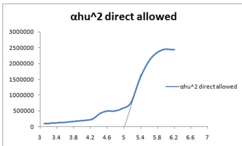
**Fig. (2) Allowed direct transition  $(ah\nu)^2$  Vs. Energy for the sample P1.**
