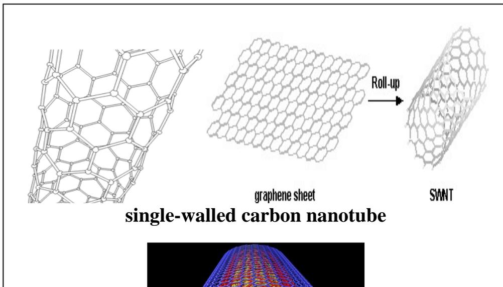
Fig .2 single-walled carbon nanotube and Multi-walled carbon nanotube [8]
