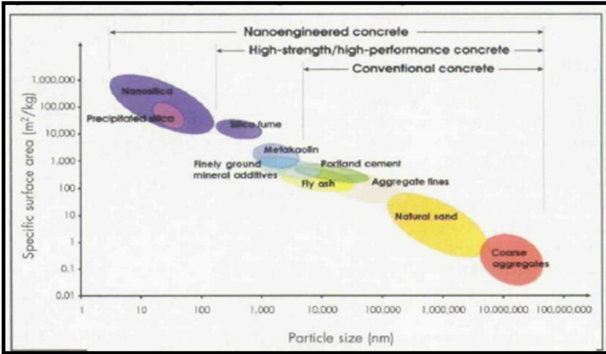
Fig .1 particle –size and specific –surface-area related to concrete materials [3]
