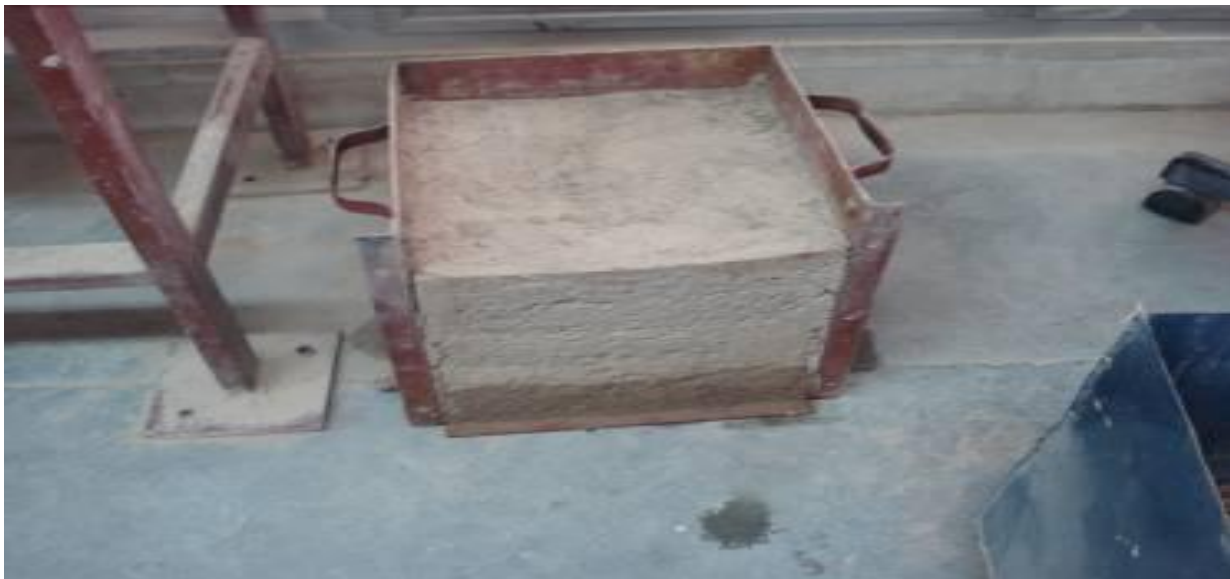
Plate 9. Effect of hydraulic conductivity of asphalt stabilized soil on capillary rise of water after static loading application.
