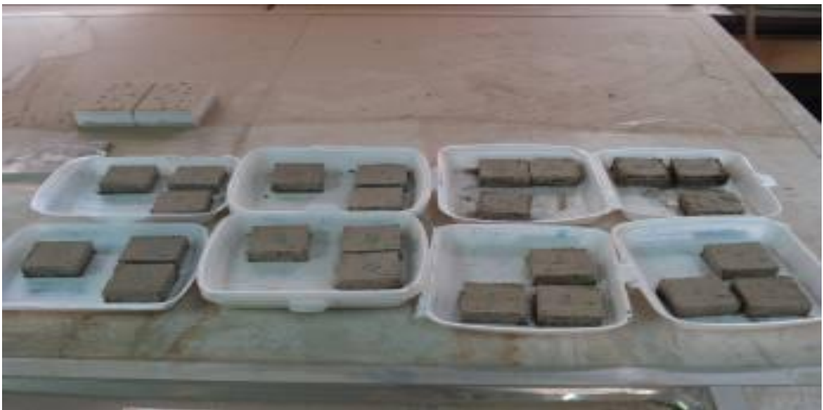
Plate 4. Curing for specimens of soil stabilized.
