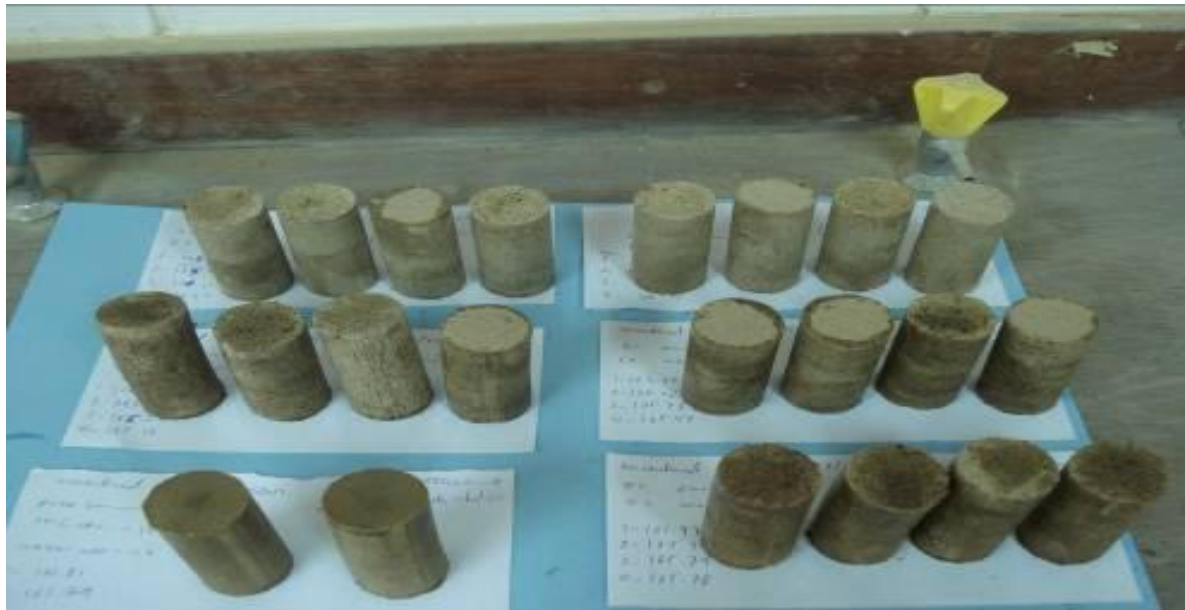
Plate 1. Curing for specimens of soil stabilized with emulsion.
