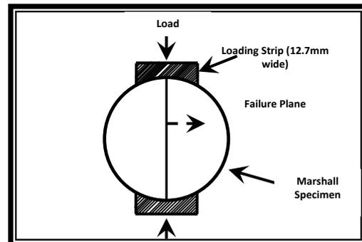
**Fig. 1:** Indirect Tensile test during Loading and at Failure
