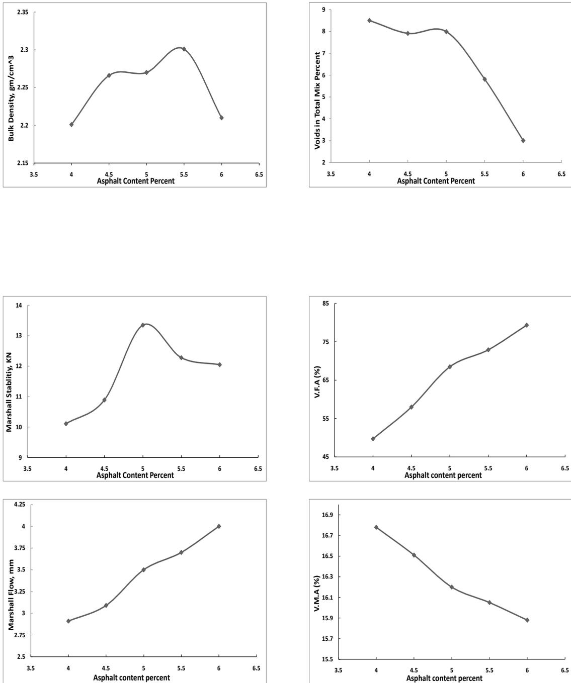
**Fig. 4** Influence of Asphalt Content on Marshall Test Properties at 50% of Recycle Concrete Mix.
