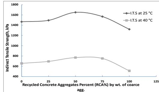
Fig. 7 Effect of Recycled Concrete Percent on Indirect Tensile Strength.
