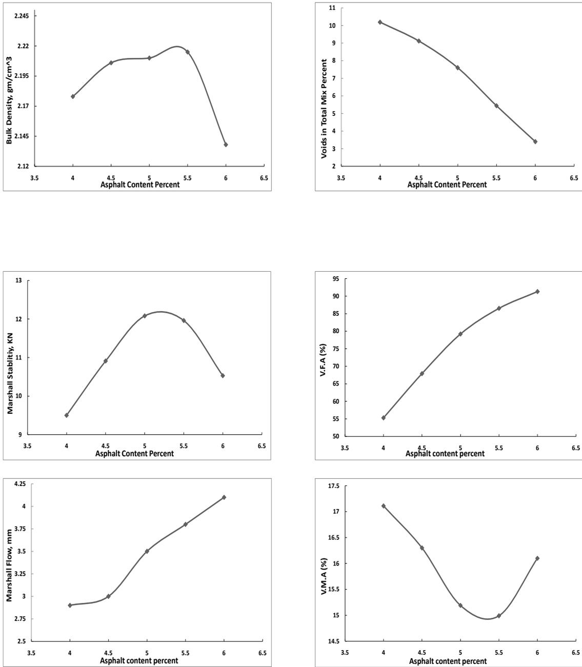
**Fig. 5** Influence of Asphalt Content on Marshall Test Properties at 75% of Recycle Concrete Mix.
