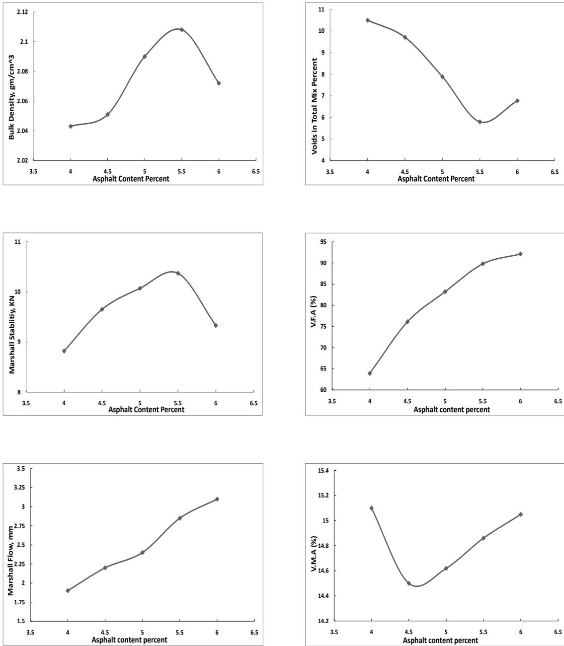
**Fig. 6:** Influence of Asphalt Content on Marshall Test Properties at 100% of Recycle Concrete Mix.
