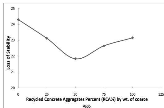
Fig.9 Effect of Recycled Concrete Percent on Loss of Stability
