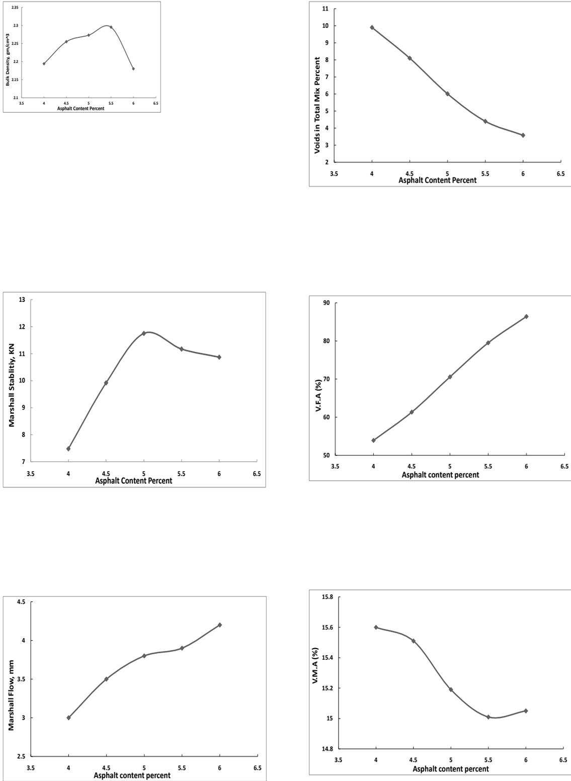
**Fig. 3** Influence of Asphalt Content on Marshall Test Properties at 25% of Recycle Concrete Mix.
