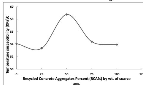
Fig.8 Effect of Recycled Concrete Percent on Temperature Susceptibility
