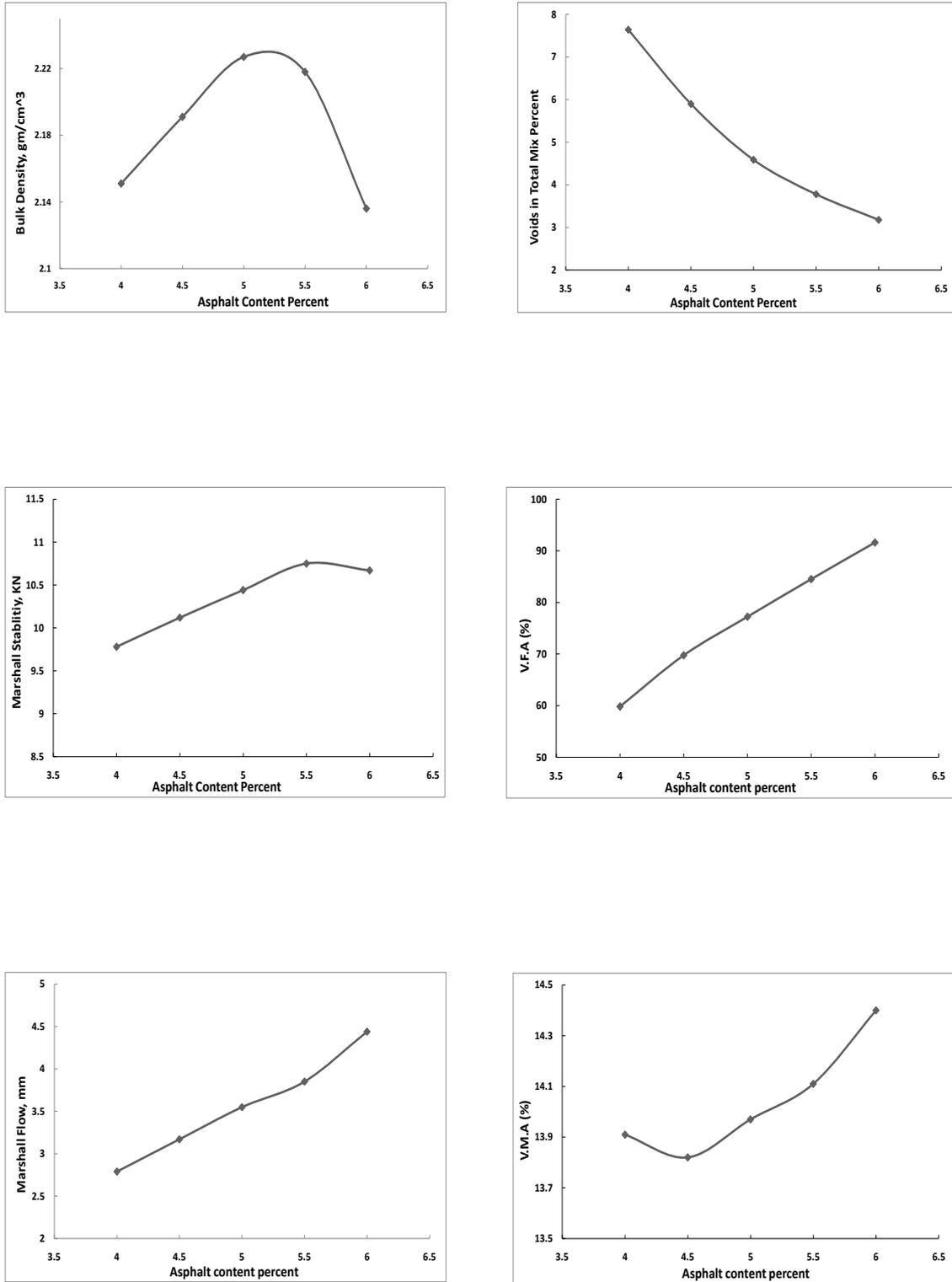
**Fig.2:**Influence of Asphalt Content on Marshall Test Properties at 0% of Recycle Concrete Mix.
