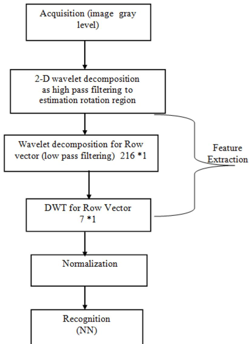
**Fig .(1): Block diagram of fingerprint recognition algorithm**
