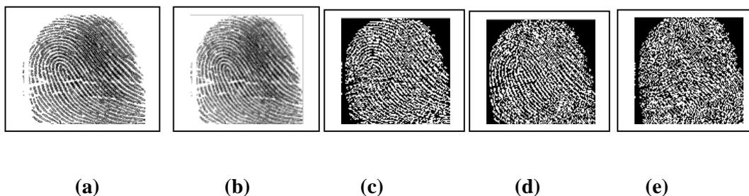
**Fig.(2): (a) Original Image (b) approximate band (LL), (c) Horizontal Subimage(HH), (d) Vertical Subimage (HV), (e) Diagonal Subimage (HD).**
