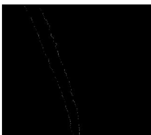
Figure-7: Edge detection using LOG operator.
