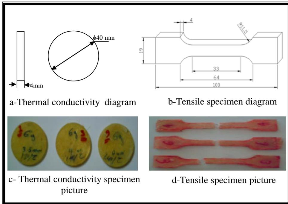
Fig. 1-a,b,c and d . The standard thermal conductivity test and tensile test specimen [7].
