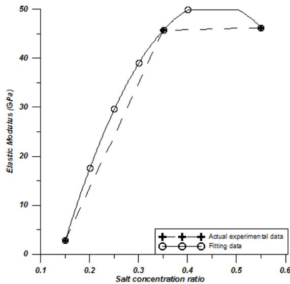
Fig. 2 . The experimental results showing the effect of salt concentration ratio on Young's Modulus
