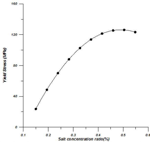
Fig. 3 . The experimental results showing the effect of salt concentration ratio on yield stress
