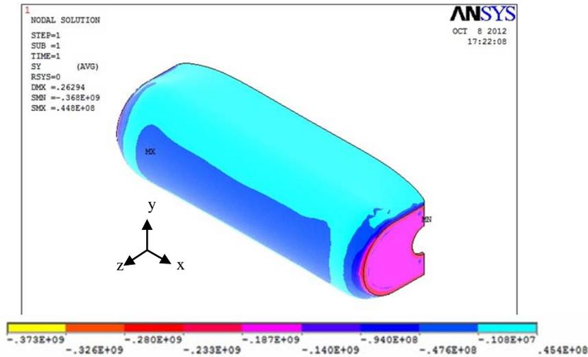
**Fig. 9. Thermal stress in y-axis direction ( $\sigma_y$ ) of composite exhaust tube in salt concentration of 35% and  $T=100\text{ C}^\circ$**
