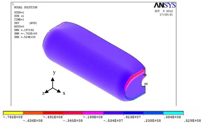
**Fig. 14. Thermal shear stress ( $\tau_{xy}$ ) of composite exhaust tube in salt concentration of 15% and  $T=100\text{ C}^{\circ}$**
