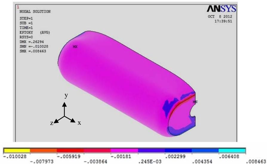
Fig. 19. Thermal shear strain ( $\gamma_{xy}$ ) of composite exhaust tube in salt concentration of 55% and T=100 C°
