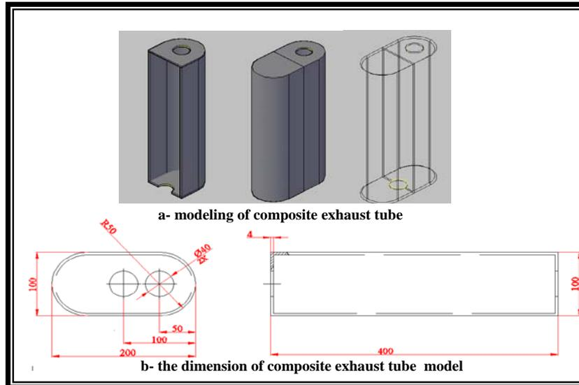
Fig .4-a, b . AutoCAD modeling and dimensions of composite exhaust tube of car
