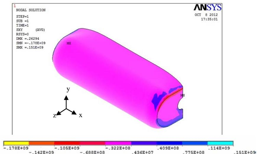
**Fig. 16. Thermal shear stress ( $\tau_{xy}$ ) of composite exhaust tube in salt concentration of 55% and  $T=100\text{ C}^{\circ}$**
