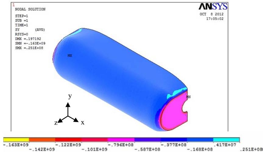
**Fig. 8. Thermal stress in y-axis direction ( $\sigma_y$ ) of composite exhaust tube in salt concentration of 15% and  $T=100\text{ C}^\circ$**
