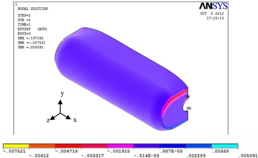
Fig. 17. Thermal shear strain ( $\gamma_{xy}$ ) of composite exhaust tube in salt concentration of 15% and T=100 C°
