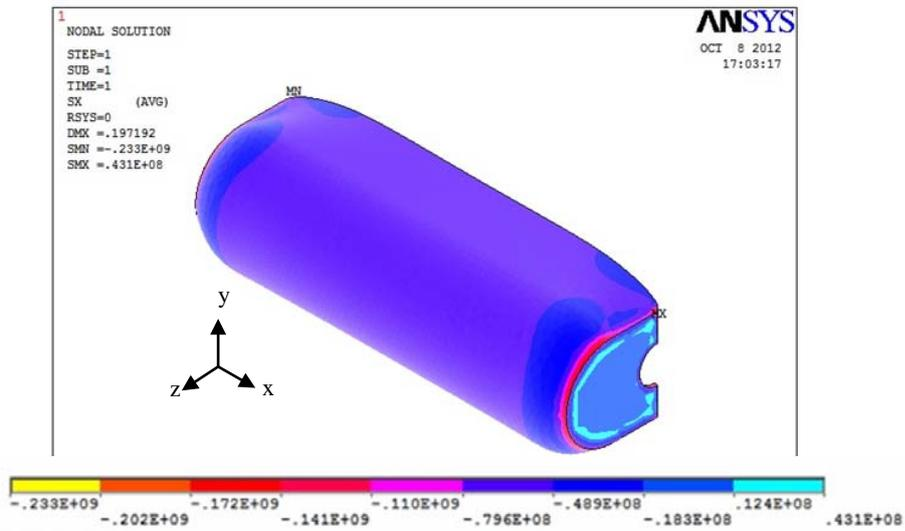
**Fig.5. Thermal stress in x-axis direction ( $\sigma_x$ ) of composite exhaust tube in salt concentration of 15% and  $T=100\text{ C}^\circ$**
