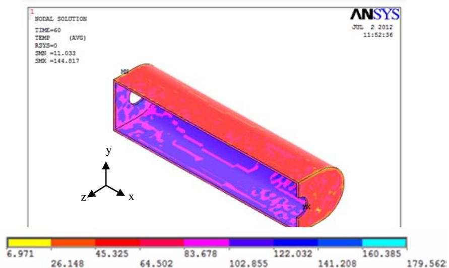
Fig. 24. The temperature distribution of composite exhaust tube of car at time of (60 sec)
