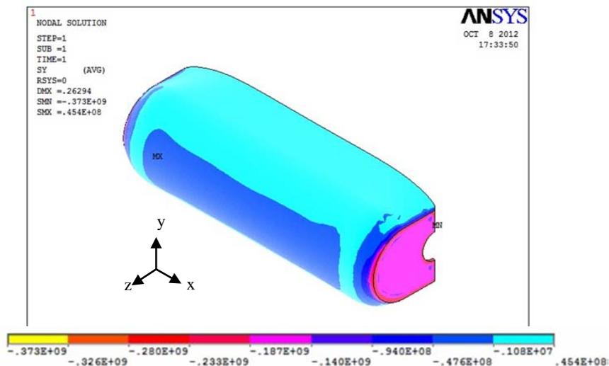
**Fig.10. Thermal stress in y-axis direction ( $\sigma_y$ ) of composite exhaust tube in salt concentration of 55% and  $T=100\text{ C}^\circ$**
