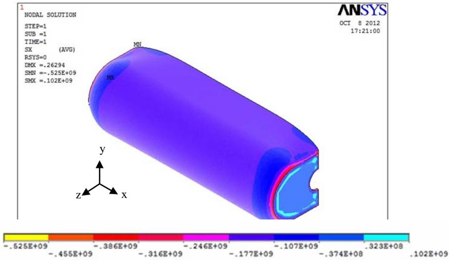
**Fig. 6. Thermal stress in x-axis direction ( $\sigma_x$ ) of composite exhaust tube in salt concentration of 35% and  $T=100\text{ C}^\circ$**
