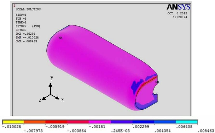
Fig. 18. Thermal shear strain ( $\gamma_{xy}$ ) of composite exhaust tube in salt concentration of 35% and T=100 C°
