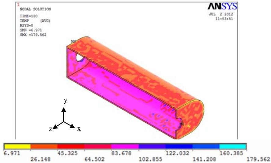
Fig. 25. The temperature distribution of composite exhaust tube of car at time of (120 sec)
