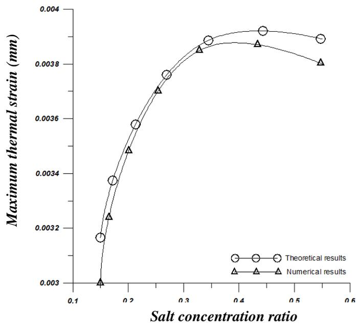
Fig. 20. The comparison between the theoretical and numerical maximum thermal strains
