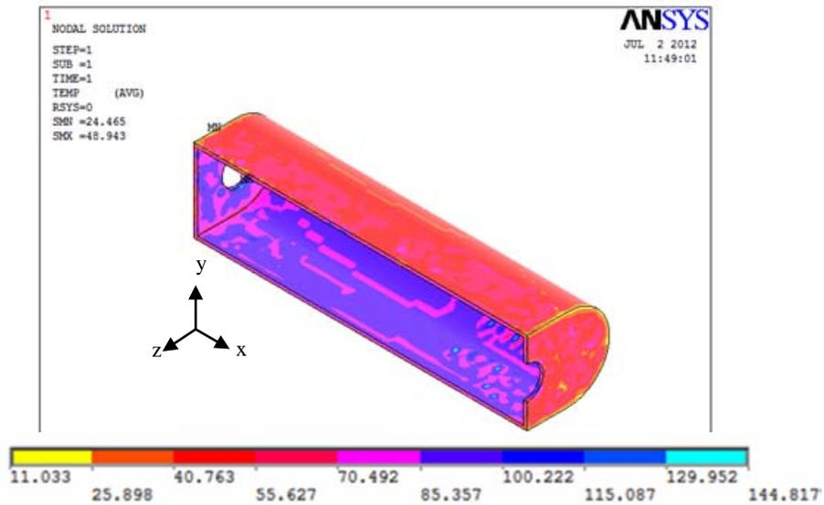
Fig. 23. The temperature distribution of composite exhaust tube of car at time of (1 sec)
