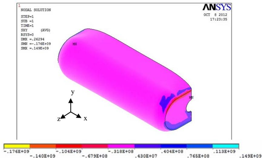
**Fig. 15. Thermal shear stress ( $\tau_{xy}$ ) of composite exhaust tube in salt concentration of 35% and  $T=100\text{ C}^{\circ}$**
