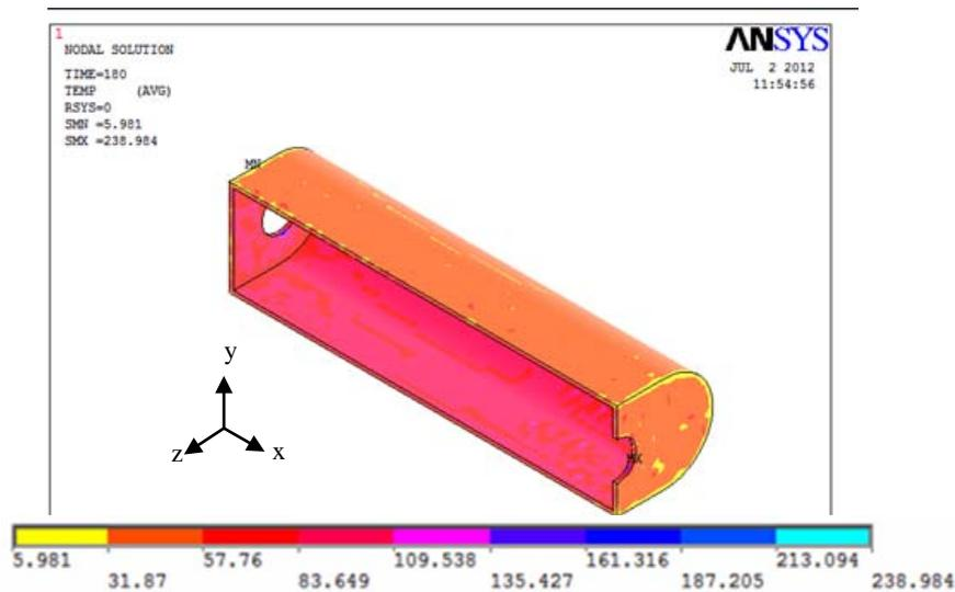
Fig. 26. The temperature distribution of composite exhaust tube of car at time of (180 sec)
