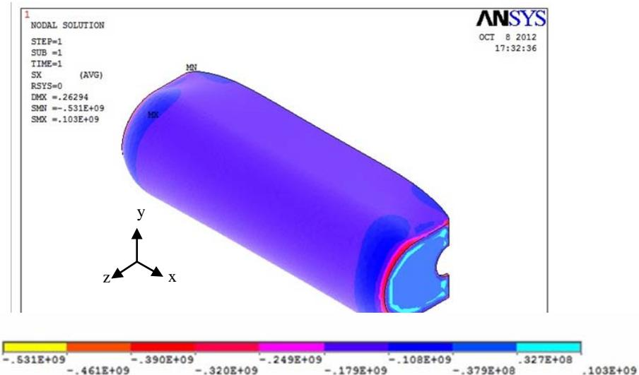
**Fig. 7. Thermal stress in x-axis direction ( $\sigma_x$ ) of composite exhaust tube in salt concentration of 55% and  $T=100\text{ C}^\circ$**
