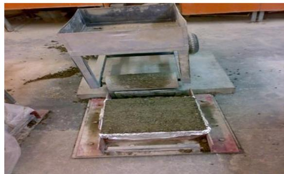
**Figure 4.** The compaction with a roller device.
