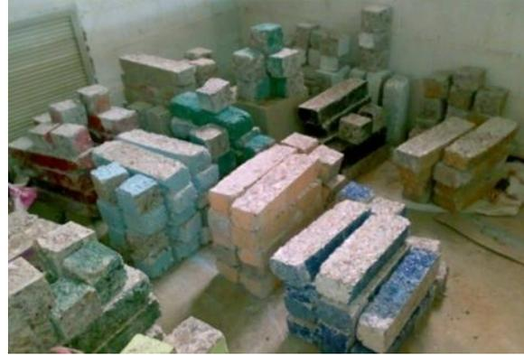
Figure 6. Part of samples obtained from RCC slab.
