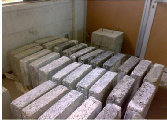
Figure 5. Part of RCC slab specimens.
