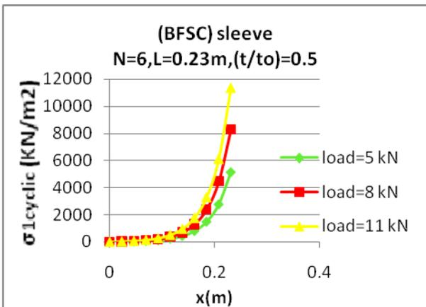
Figure 9. Principal stress distribution along a (bfsc) sleeve for 3 different cyclic loads.
