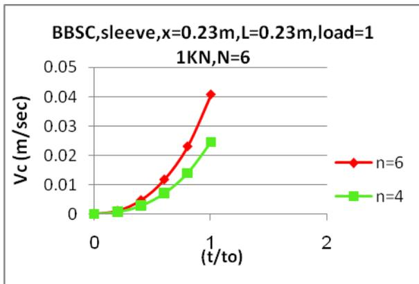
**Figure 20.** Variation of velocity of crack propagation with wave propagation time for 2 different numbers of cycles.
