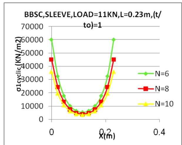
Figure 11. Stress distribution along a (bbcs) sleeve for 3 different numbers of teeth.
