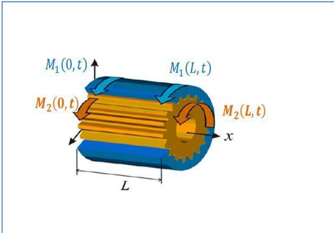
**Figure 1.** Schematic figure of the spline coupling.
