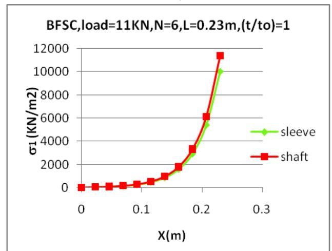
**Figure 5.** Principal stress distribution along the axial direction of a (bfsc) tooth due to impact load.
