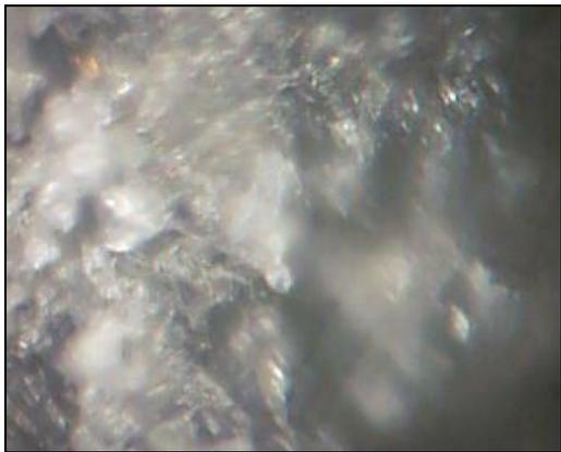
**Fig. (5) Fracture surface from left side of (UPE/PU) blend +10% volume fraction of glass powder Composite.**
