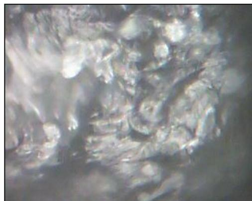
**Fig. (2) Fracture surface from right side of (UPE/PU) blend.**
