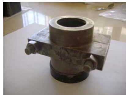
Figure (1): Special split mold for cylindrical shape specimen
