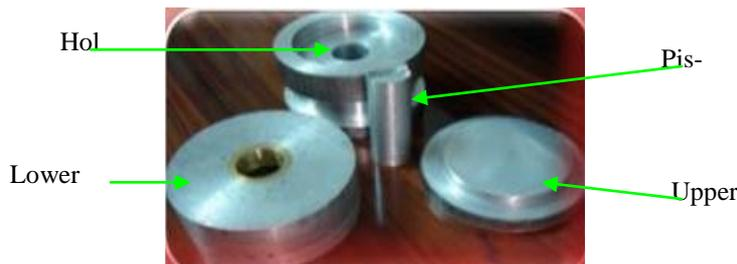
Figure (1): Metal Mold Used for Acrylic Resin Sample Discs Preparation
