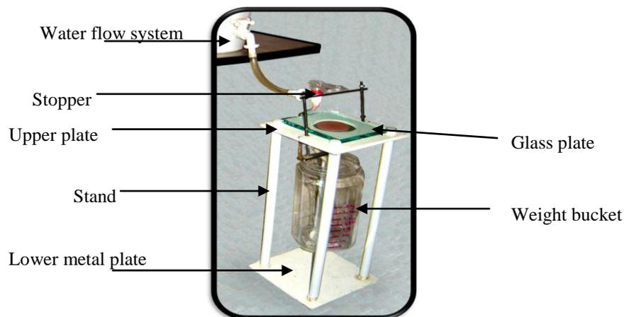
Figure (3): Testing Apparatus for Retention Test
