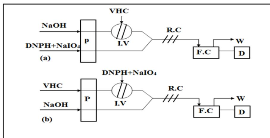
**Figure 1-** Schematic diagram of flow injection-Spectrophotometric analysis P, Peristaltic pump; I.V, Injection valve; R.C, Reaction coil; F.C, Flow cell; D, Detector (vis-spectrophotometric); W, Waste.
