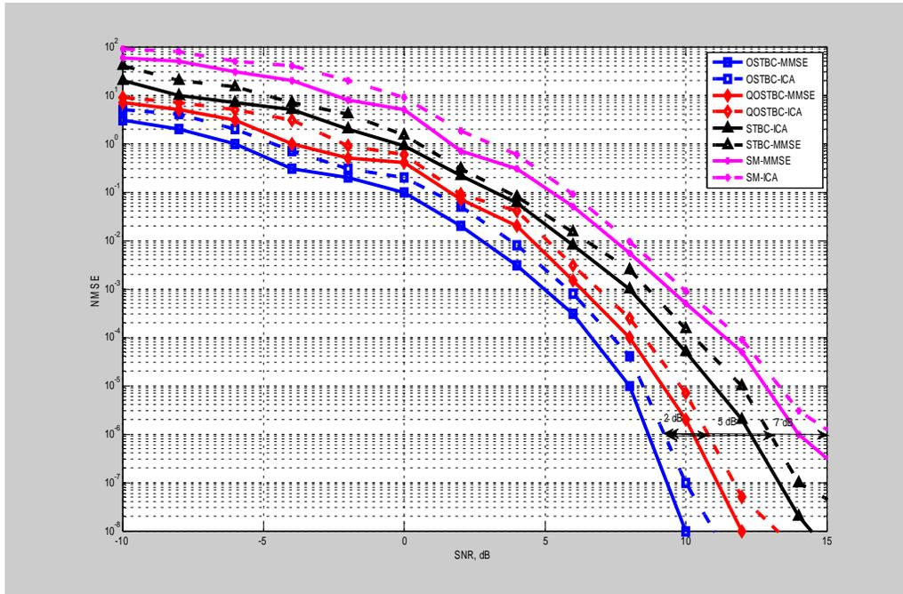
Figure (6) SNR versus NMSE Performance Comparison for ( $N_t=2, N_r=2$ ).
