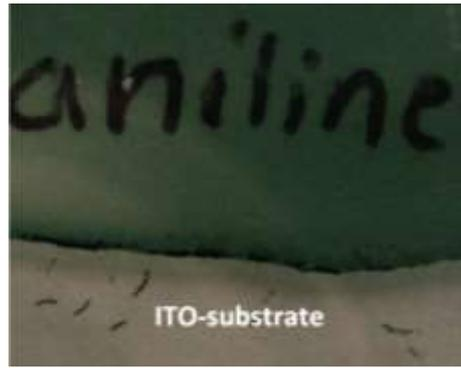
Fig. (4) Photograph of PANi film deposited on ITO
