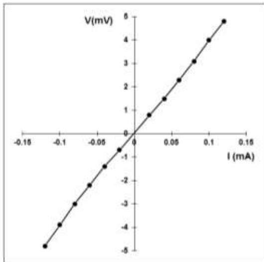
Fig. (8) I-V characteristics of PANi film deposited on ITO
