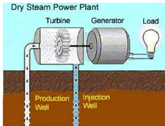
Figure 1: Block Diagram of Dry Steam Plant of Geothermal production
