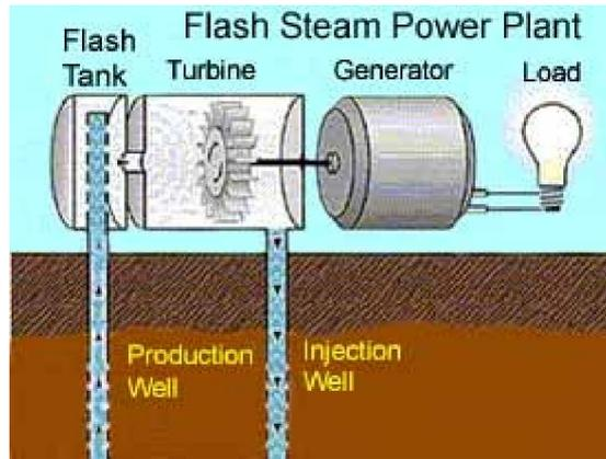
Figure 2: Block Diagram of Flash Steam Power Plant of Geothermal production
