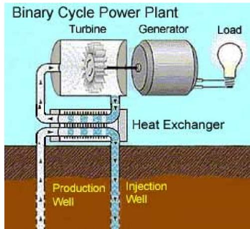
Figure 3: Block Diagram of Binary Cycle Power Plant of Geothermal production
