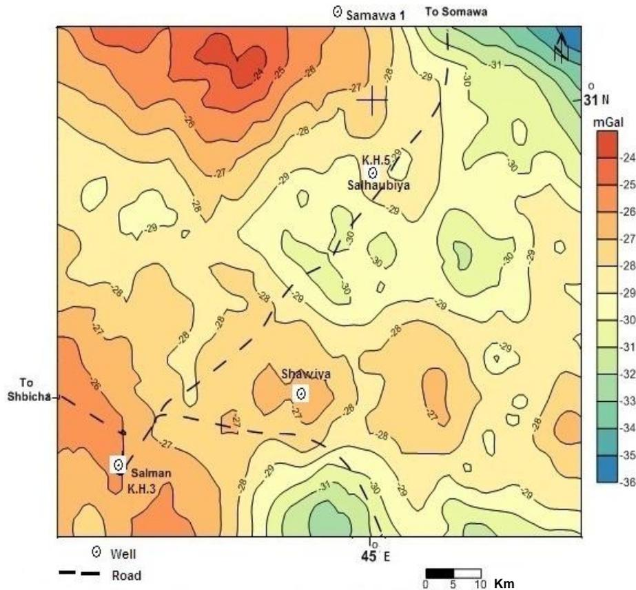
Fig.2: Observed Bouguer anomaly map with borehole locations
