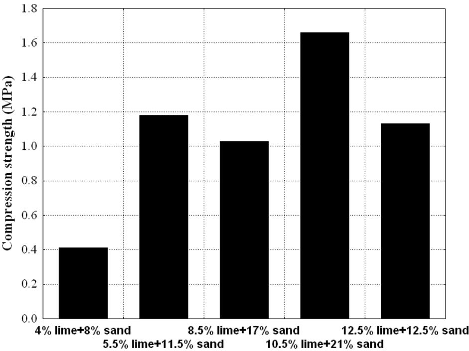
**Fig .(6): The compression strength of RAP materials plus bricks sand treated with different percentages of hydrated lime and tested after 7 of curing in air.**
