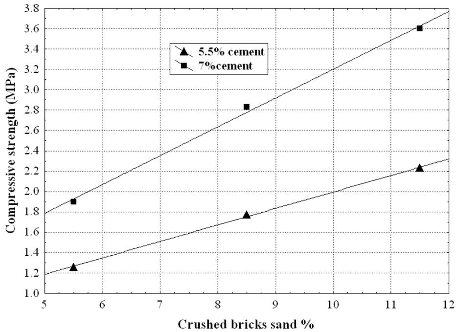
**Fig .(8):** The compression strength of RAP materials plus bricks sand treated with two percentages of Portland cement and tested after 7 of curing in water.
