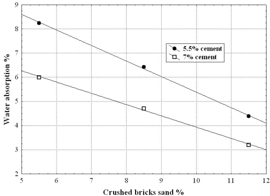
**Fig .(10): The water absorption of RAP materials plus bricks sand treated with two percentages of Portland cement and tested after 7 of curing in water.**
