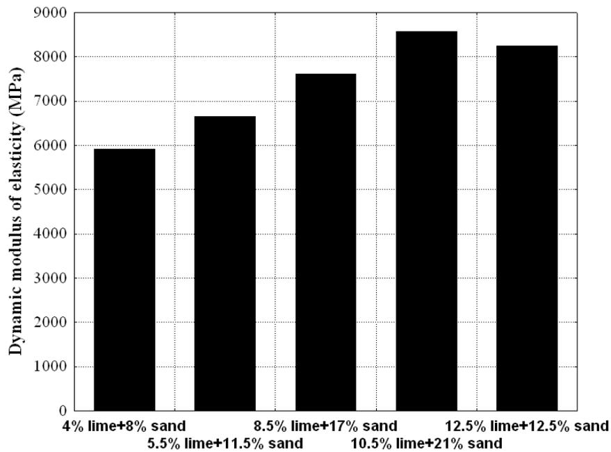
Fig.(16) The dynamic modulus of RAP materials plus bricks sand treated with different percentages of hydrated lime and tested after 7 of curing in air.
