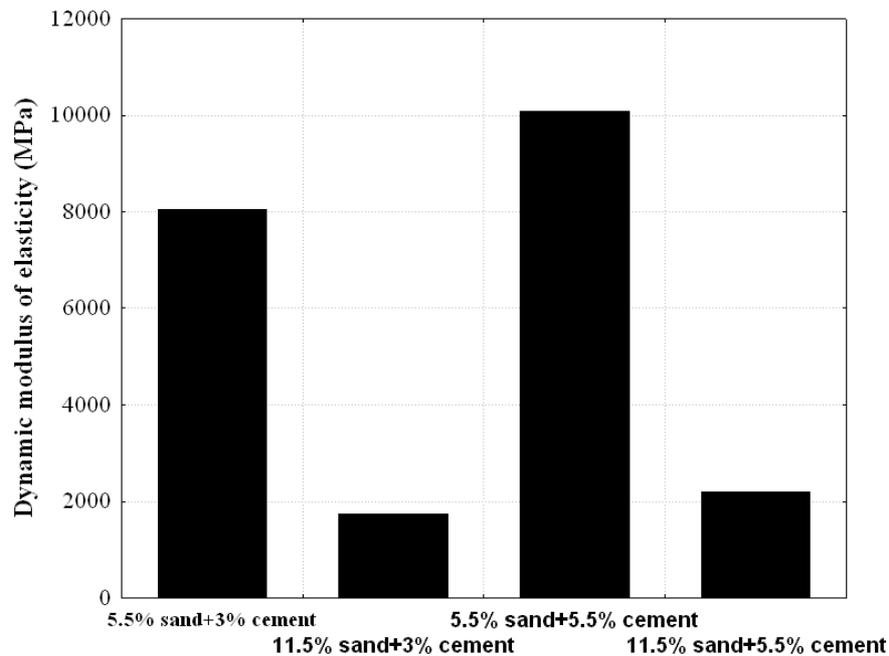
**Fig .(18) The dynamic modulus of RAP materials plus bricks sand treated with different percentages of Portland cement and 5.5% hydrated lime and tested after 7 of curing in air.**
