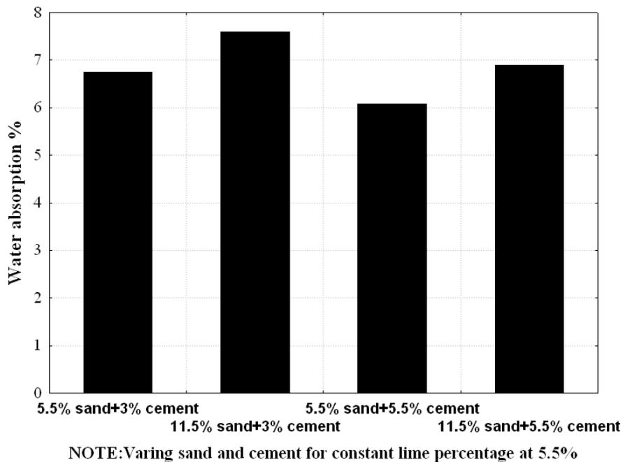
**Fig .(14) The water absorption of RAP materials plus bricks sand treated with different percentages of Portland cement and 5.5% hydrated lime and tested after 7 of curing in water.**
