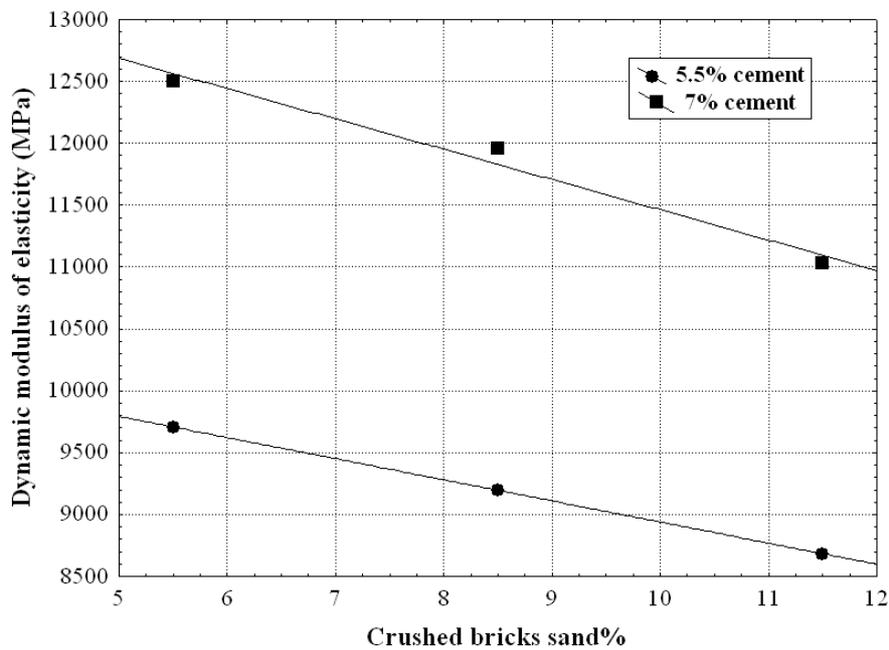
Fig.(17) The dynamic modulus of RAP materials plus bricks sand treated with different percentages of Portland cement and tested after 7 of curing in water.
