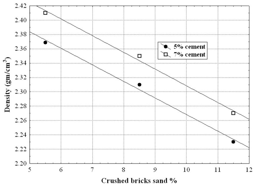
**Fig .(9)** The density of RAP materials plus bricks sand treated with two percentages of Portland cement and tested after 7 of curing in water.
