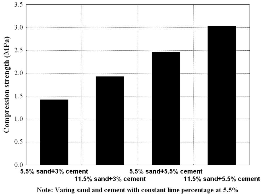
**Fig .(11) The compressive strength of RAP materials plus bricks sand treated with different percentages of Portland cement with 5.5% hydrated lime and tested after 7 of curing in air.**
