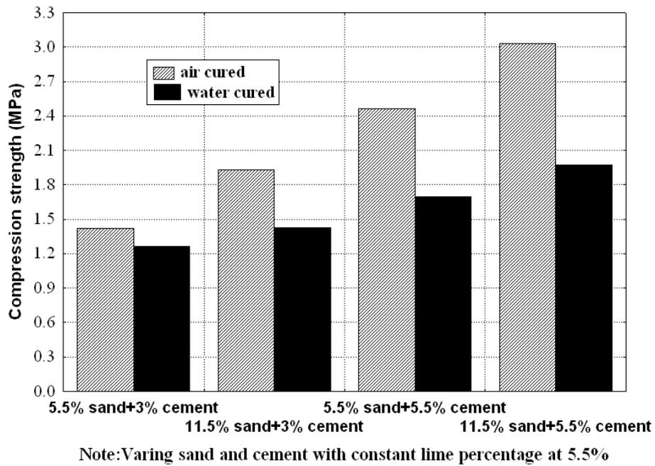
**Fig .(13) The compression strength of RAP materials plus bricks sand treated with different percentages of Portland cement and 5.5% hydrated lime and tested after 7 of curing in air and in water.**
