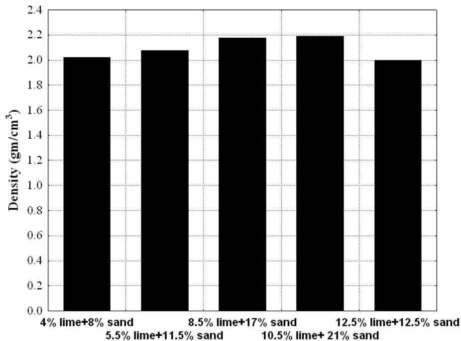
**Fig .(7): The density of RAP materials plus bricks sand treated with different percentages of hydrated lime and tested after 7 of curing in air**
