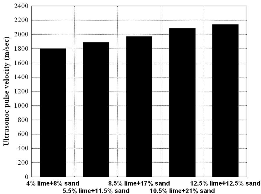
**Fig .(15) The ultrasonic pulse velocity of RAP materials plus bricks sand treated with different percentages of hydrated lime and tested after 7 of curing in air.**
