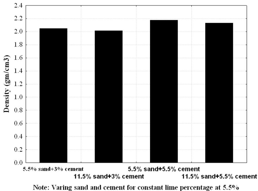
**Fig .(12) The density of RAP materials plus bricks sand treated with different percentages of Portland cement and 5.5% hydrated lime and tested after 7 of curing in air.**
