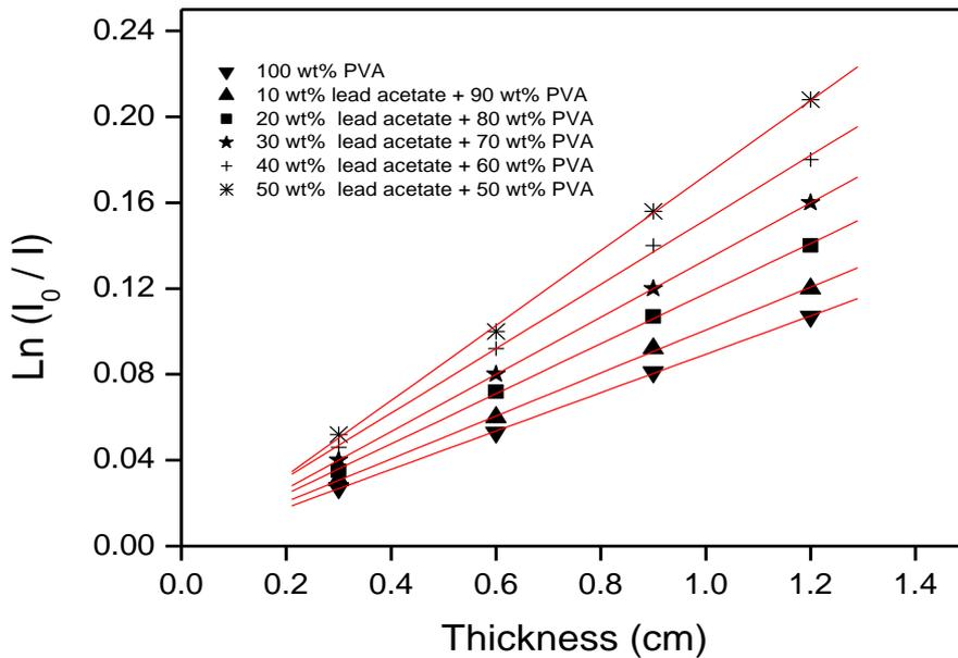
Figure 3.  $\ln(I_0/I)$  versus thickness for lead acetate-PVA polymer samples at 0.662 MeV.
