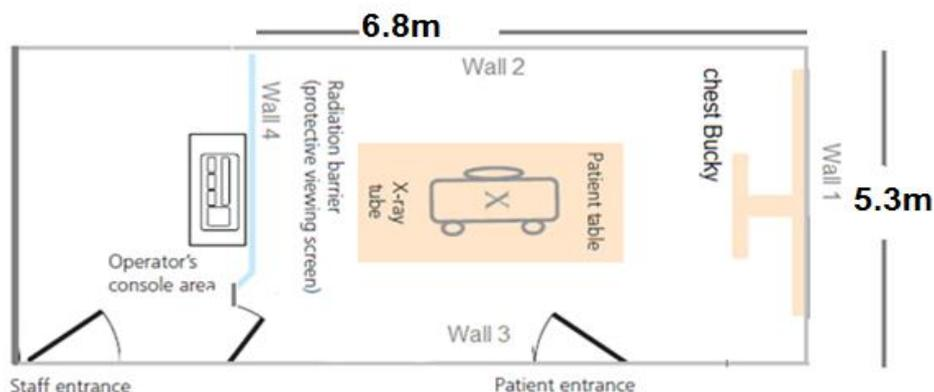
Figure 2.The geometry of chest x-ray examination room
