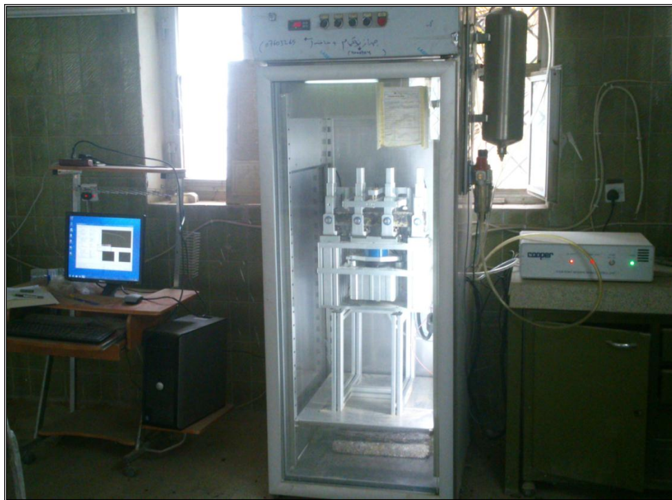
Figure 4. Flexural fatigue testing equipment (NCCLR laboratory, Baghdad).
