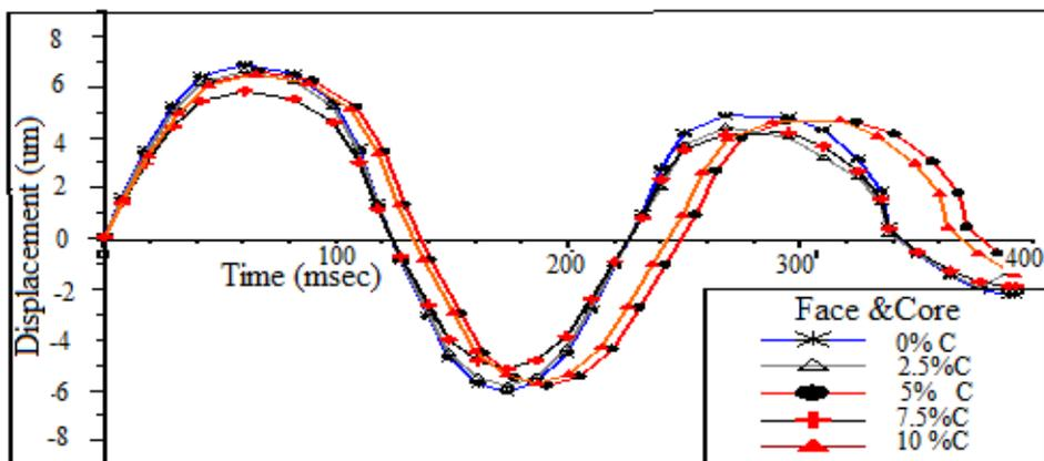
Fig .(7) Effect of graphite filler content on the deflection behavior of honey comb sandwich panel at (m=80g & h= 90cm).
