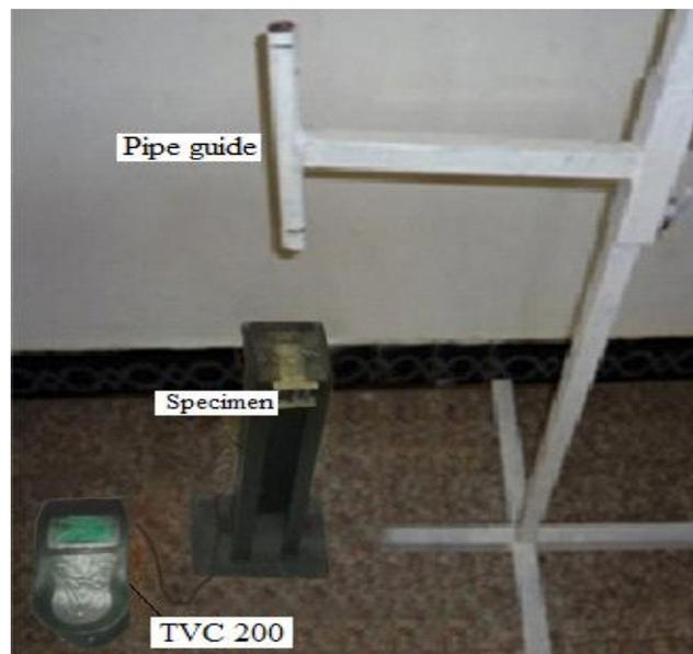
**Fig .(3) The dynamic response test rig.**
