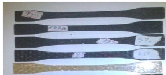
Fig .(2) The Tensile test specimens according to (ASTM D-638) [7].
