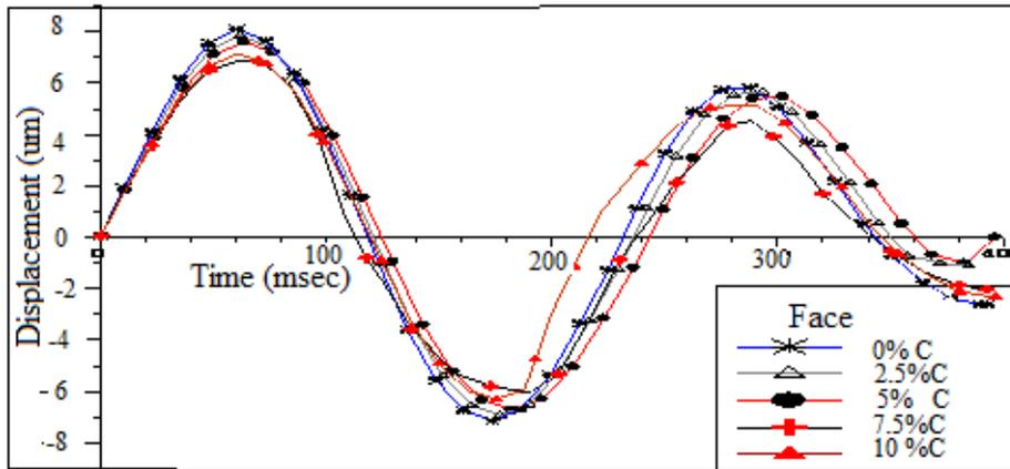
Fig .(9) The defection behavior of honey comb with different faces and 0% C core at (m=80g & h=120cm).
