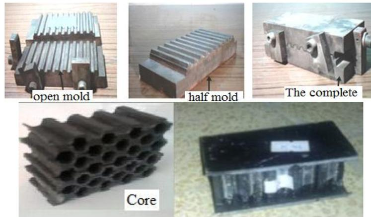
Fig .(1) The Honey comb mold and sandwich panel.
