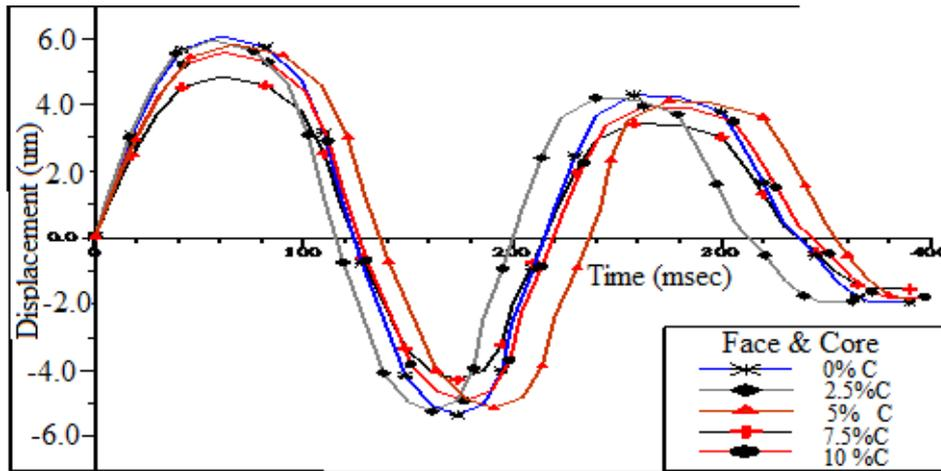
Fig .(5) Effect of graphite filler content on the deflection behavior of honey comb sandwich panel at (m=45g & h=90cm).
