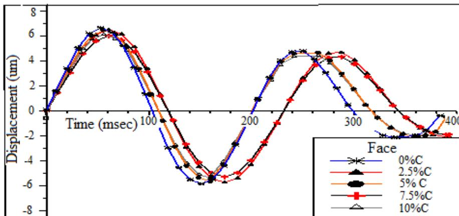
Fig .(13) The defection behavior of honey comb with different faces and 10% C core at (m=80g & h=120cm).
