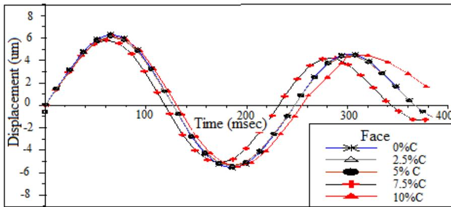
Fig .(12) The defection behavior of honey comb with different faces and 7.5% C core at (m=80g & h=120cm).
