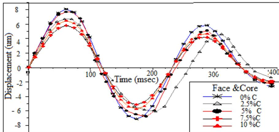
**Fig .(8) Effect of graphite filler content on the deflection behavior of honey comb sandwich panel at (m=80g & h=120cm).**
