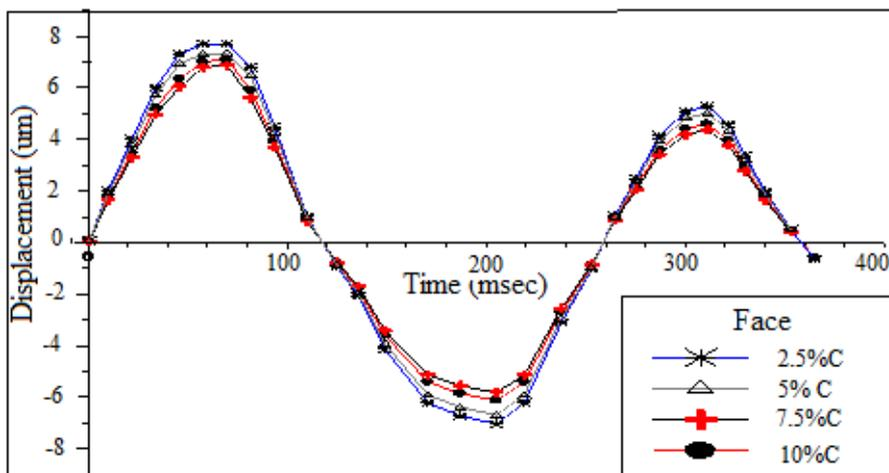
Fig .(11) The defection behavior of honey comb with different faces and 5% C core at (m=80g & h=120cm).
