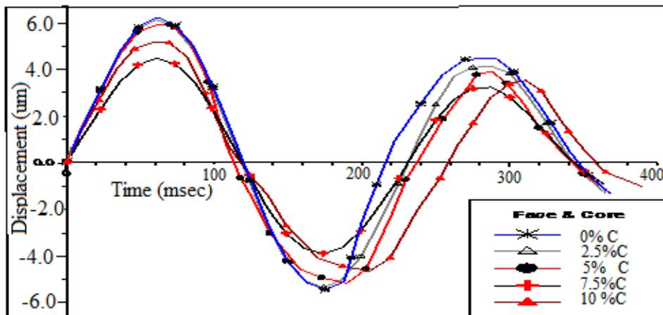
Fig .(6) Effect of graphite filler content on the deflection behavior of honey comb sandwich panel at (m=45g & h=120cm).
