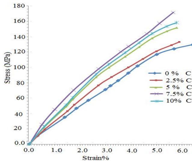
**Fig .(4) Effect of graphite filler content on the Stress-strain behavior of tensile test.**
