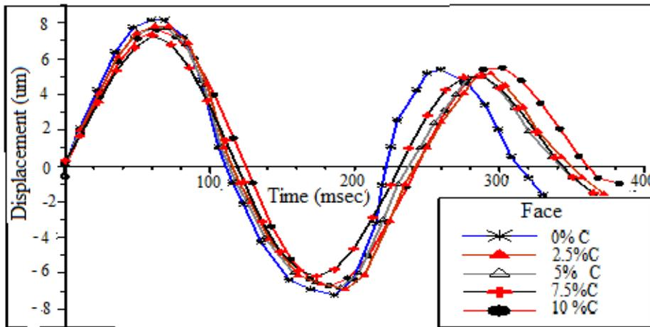
Fig .(10) The defection behavior of honey comb with different faces and 2.5% C core at (m=80g & h=120cm).
