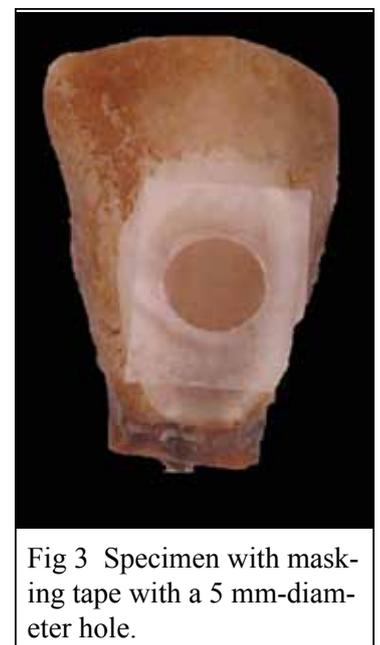
Fig 3 Specimen with masking tape with a 5 mm-diameter hole.
