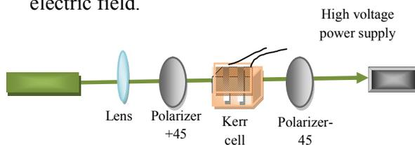
Figure 3: Experimental setup
