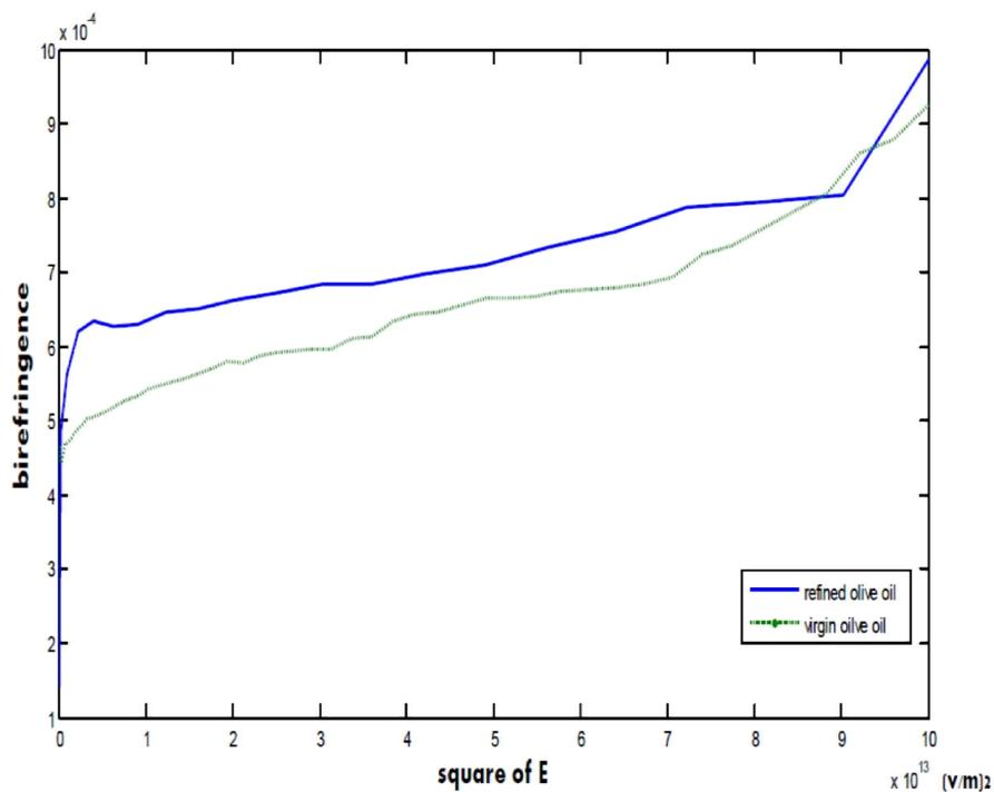
Figure 5: The birefringence  $\Delta n$  versus Square of applied electric field using 660nm.
