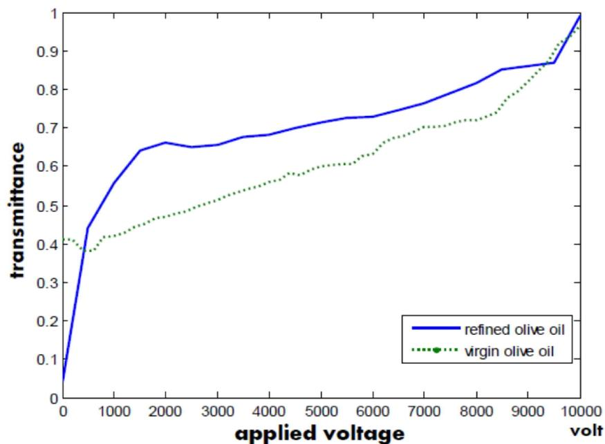
Figure 4: The transmittance of virgin and refined olive oil versus the applied voltage at 660nm.
