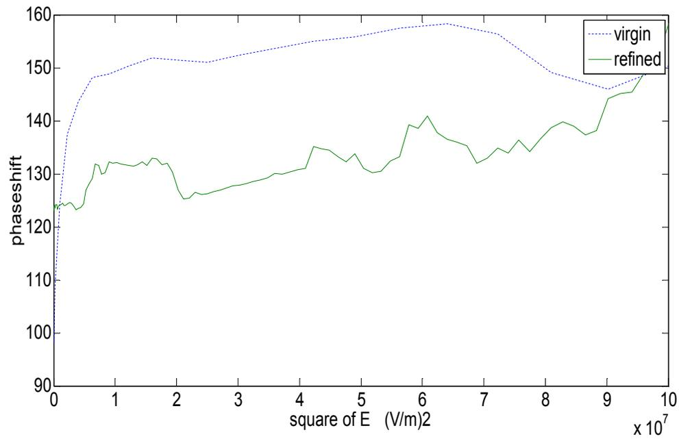
Figure 9: The phase shift versus Square of applied electric field using 532nm.
