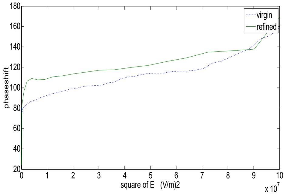
Figure 8: The phase shift versus Square of applied electric field using 660nm.
