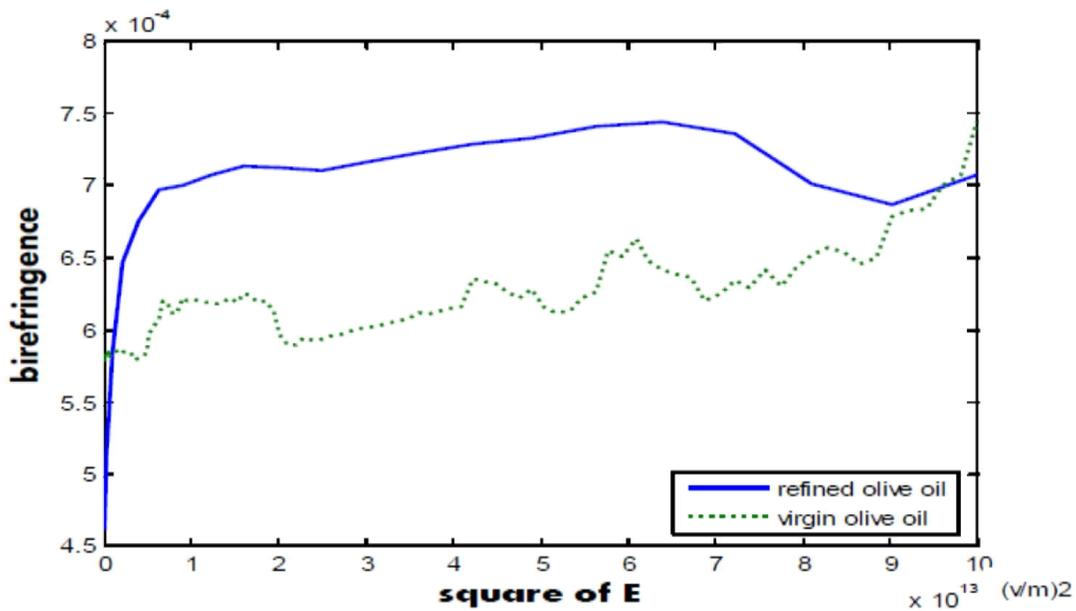
Figure 7: The birefringence  $\Delta n$  versus Square of applied electric field using 532nm.
