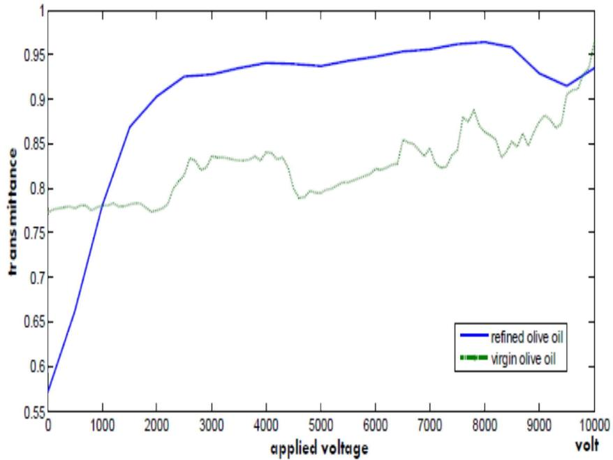
Figure 6: The transmittance of virgin and refined olive oil versus the applied voltage at 532nm.
