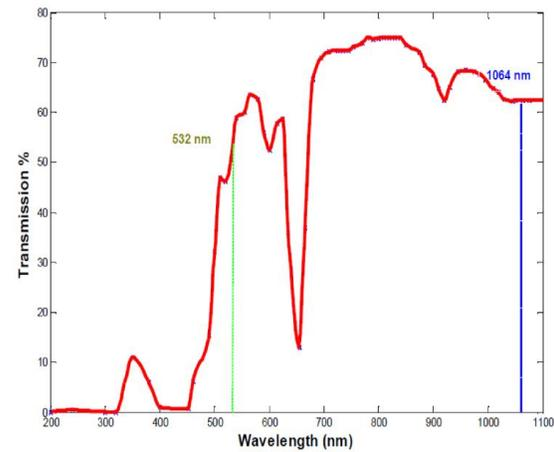
**Figure 1: UV-VIS transmission of olive oil**
