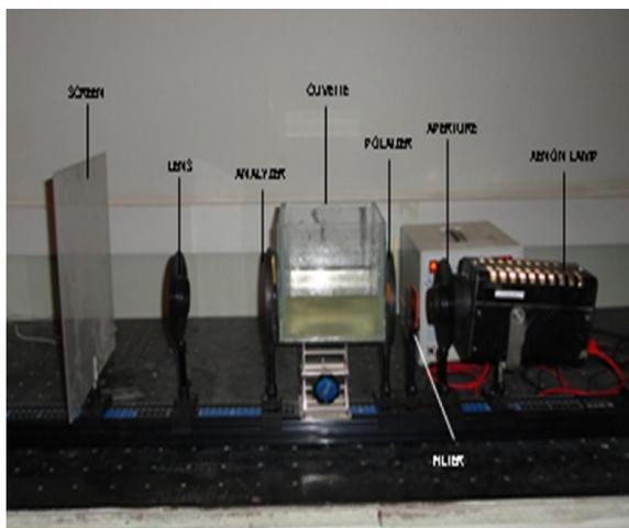
**Figure 1(a) First experimental setup with xenon lamp.**
