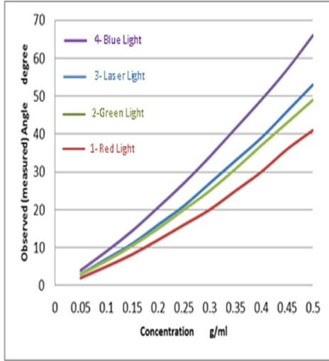
**Figure 2: Observed Angle versus concentration at different light sources**
