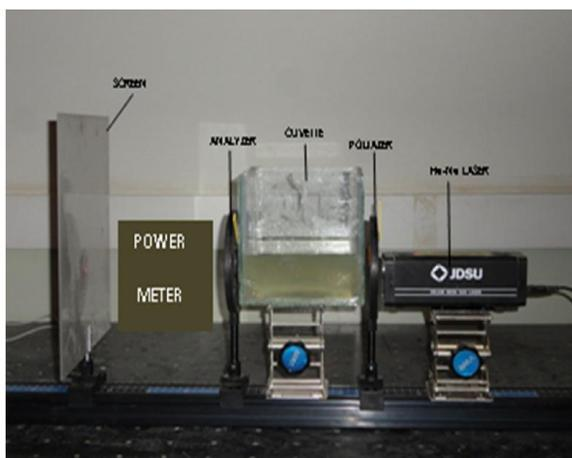
**Figure 1(b) Second experimental setup with laser beam.**
