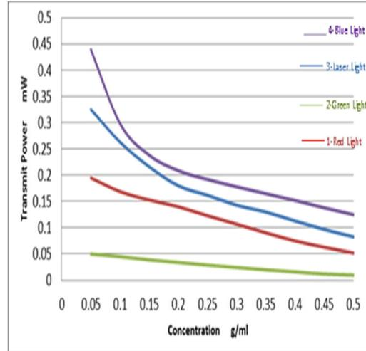
**Figure 4: Transmitted power versus concentration at different light sources**
