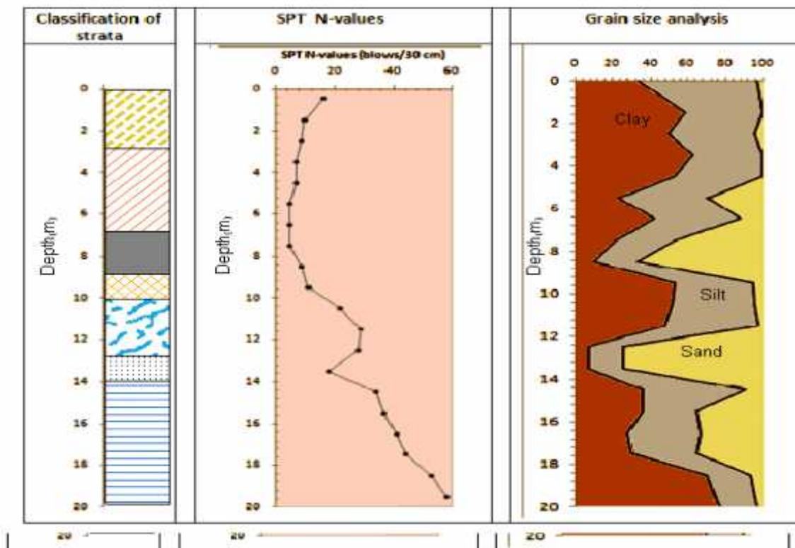
Figure 6: Bearing strata, N-values and grain size analysis of soils at Al-Maymonah (Site 5)
