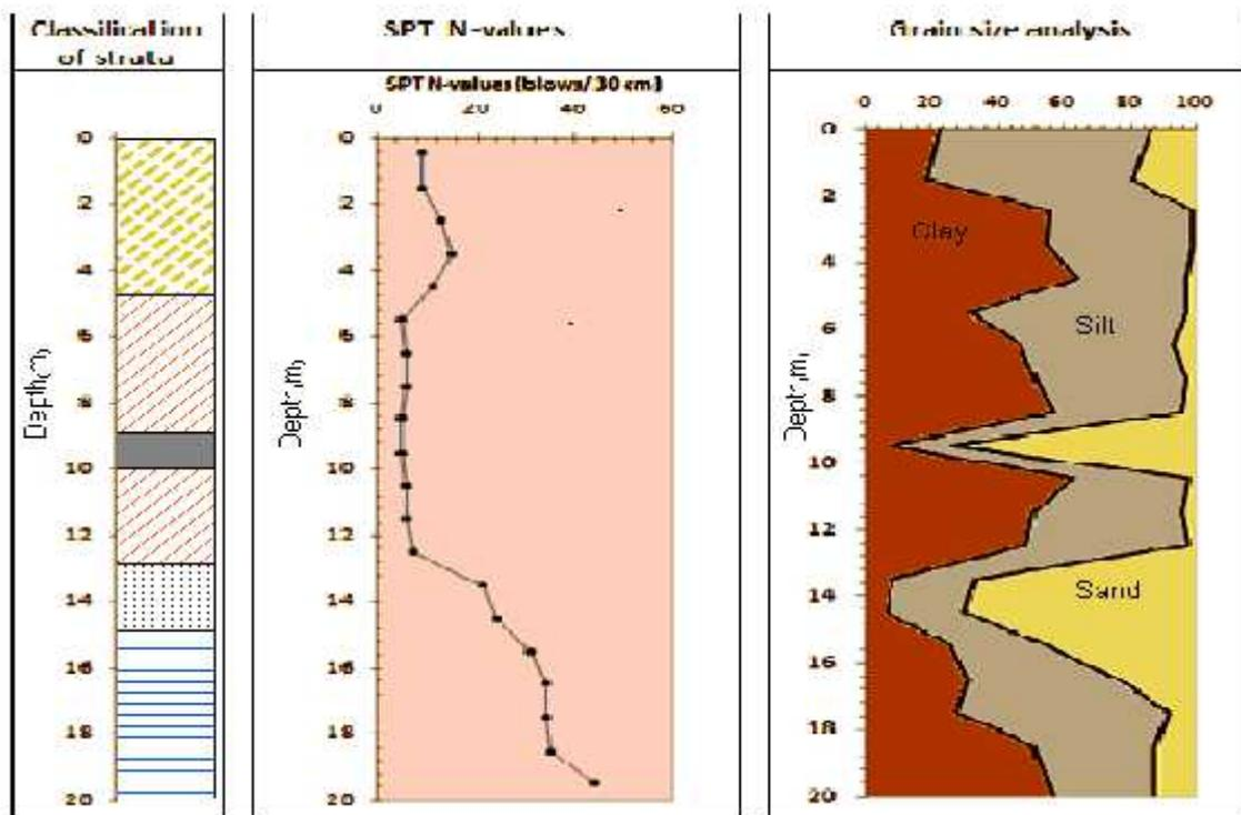
**Figure 8:** Bearing strata, N-values and grain size analysis of soils at Kalat Salih(Site 7)
