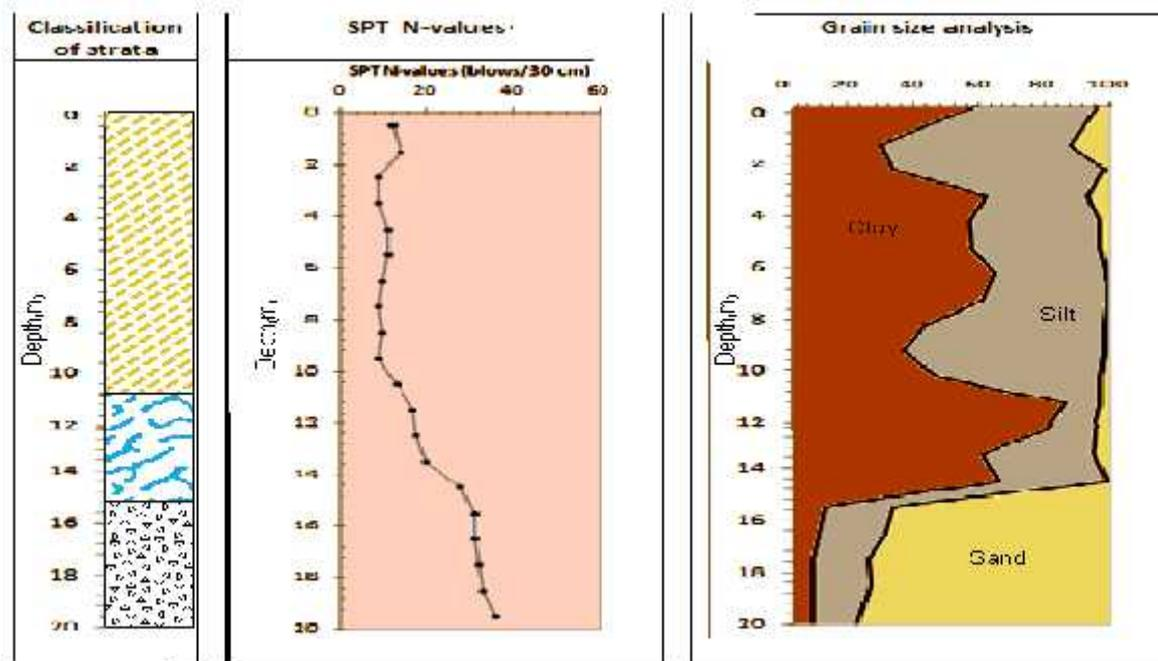
**Figure 4:** Bearing strata, N-values and grain size analysis of soils at Al-Umara dam (Site 3)
