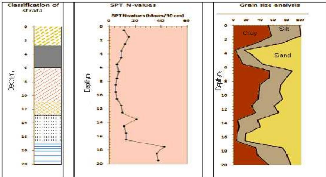
**Figure 7:** Bearing strata, N-values and grain size analysis of soils at Al- Kahlaa (Site 6)
