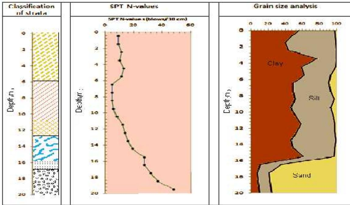
**Figure 3:** Bearing strata, N-values and grain size analysis of soils at Umara city (Site 2)
