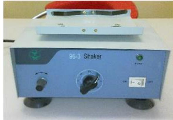
Figure (2): electrical vibrator
