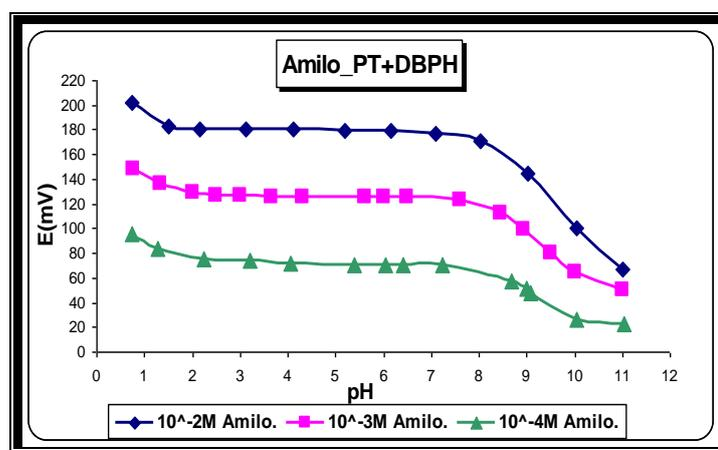
Fig.-5: Effect of pH on the potential of the electrode A (Amilo-PT+DBPH) at concentrations 10<sup>-2</sup>, 10<sup>-3</sup> and 10<sup>-4</sup> M.
