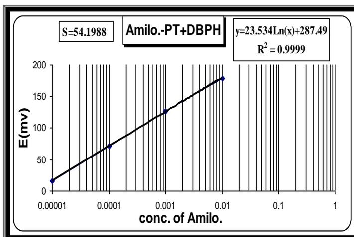
Fig.-7: Calibration curve of electrode A (Amilo-PT+DBPH).
