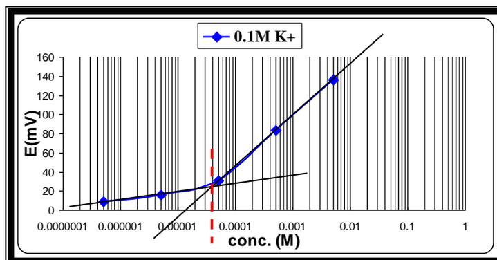
Fig.-6: FIM calibration curve for electrode A (Amilo-PT+DBPH),  $K^+$  ( $5 \times 10^{-2} M$ ) as interfering ion  $a_A = 4 \times 10^{-5} M$ .
