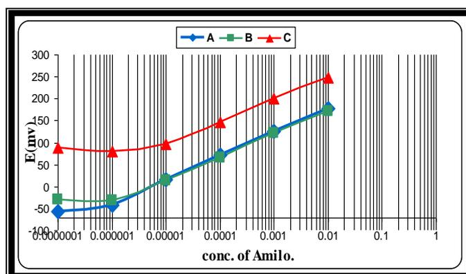
Fig.-3: Calibration curves of Amiloride hydrochloride selective electrodes (A, B and C) using (Amilo-PT) ion-pair complex.
