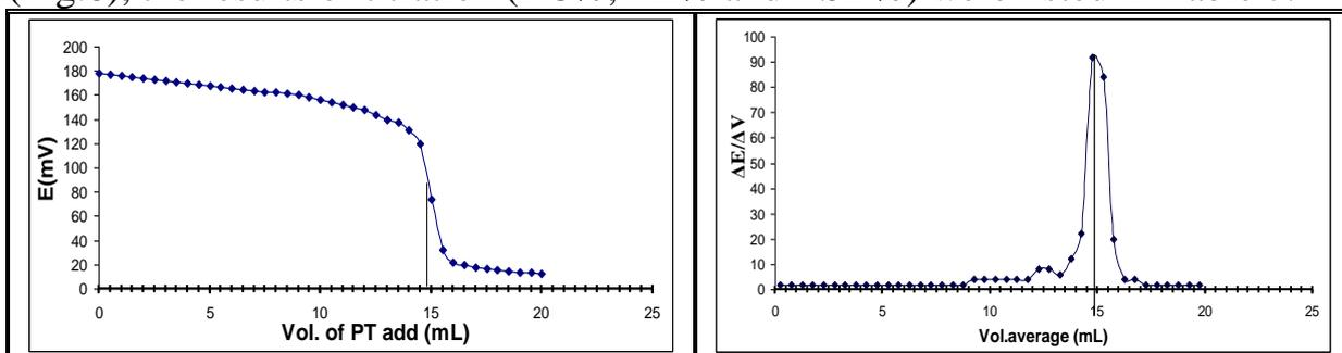
Fig.-9: Titration curve of electrode A (Amilo-PT+DBPH) for 15 mL sample solution 0.01 M Amiloride hydrochloride with 0.01 M of PT as a titrant solution.
