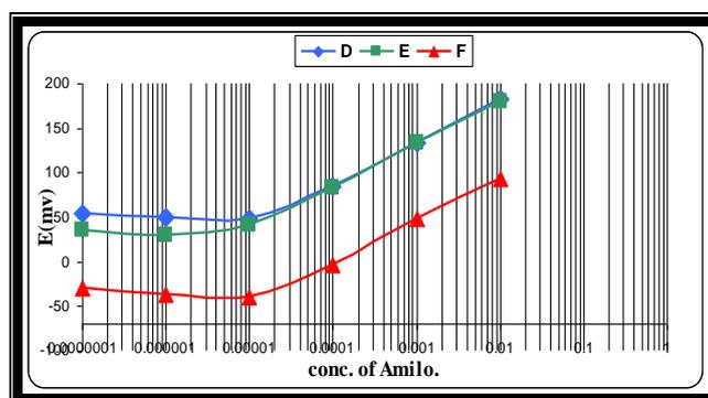
Fig.-4: Calibration curves of Amiloride hydrochloride selective electrodes (D, E and F) using (Amilo-TPB) ion-pair complex.
