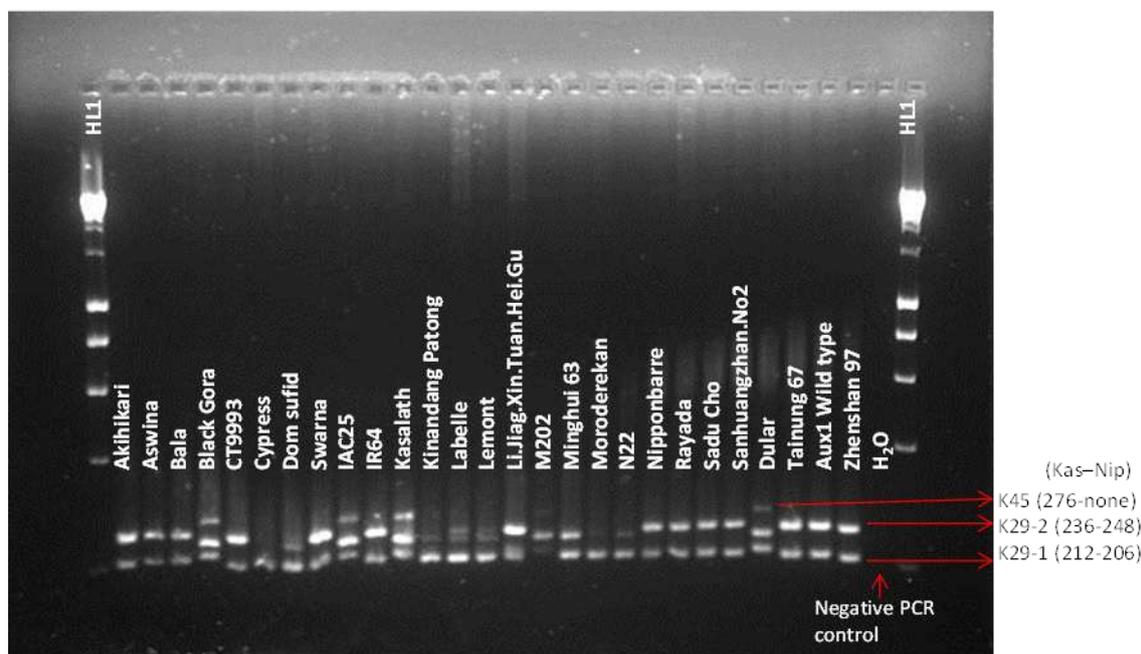
**Figure 2. Testing 27 genotypes on a 3 % agarose gel with three markers K45, K29-1 and K29-2 (see Table 1 for primer sequence). HL1= Hyper Ladder 1 DNA size marker (Bioioine, UK)**
