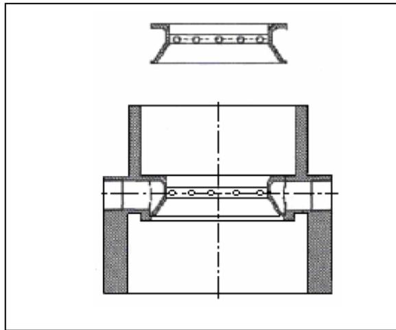
*Fig. 2 The Cross Sectional Drawing of the Mixer*
