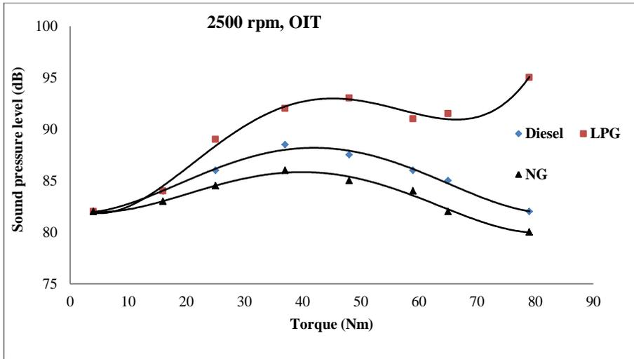
Fig. 9, The Effect Of Load On Noise Levels For Variable Fuels At Constant High Engine Speed And Optimum Injection Timing.
