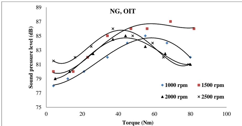
*Fig. 7, the Effect of Load on Noise Levels For Duel Fuel (Diesel+NG) At Variable Engine Speed and Optimum Injection Timing*
