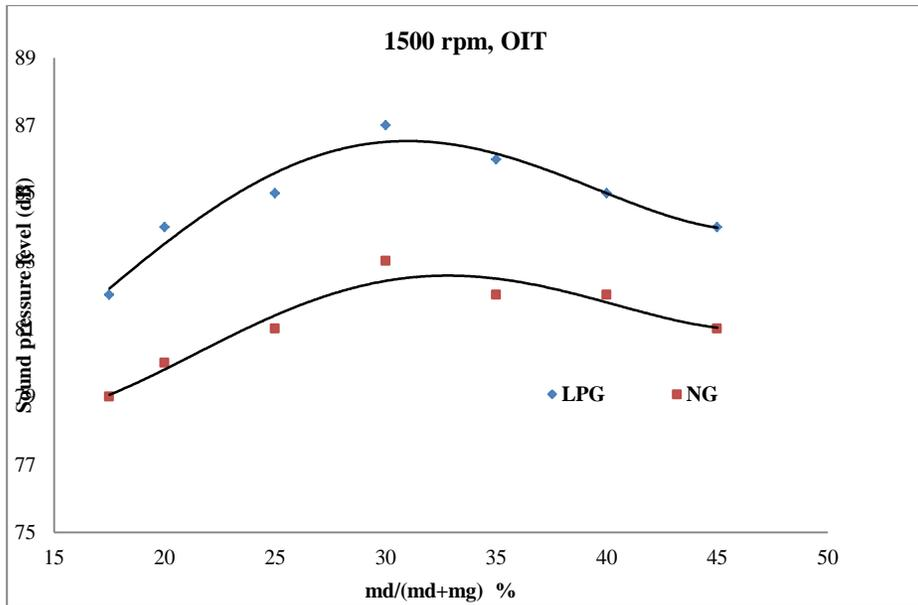
*Fig. 11, The Effect Of Pilot Fuel Percentage On Noise Levels For Variable Fuels At Constant Engine Speed.*
