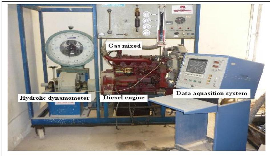
*Fig. 3 Photographic Picture of the Testing Rig*
