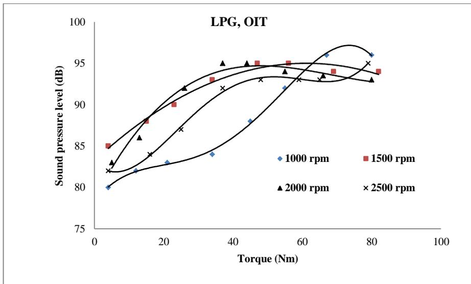
*Fig. 8, the Effect of Load on Noise Levels For Duel Fuel (Diesel+LPG) At Variable Engine Speed and Optimum Injection Timing*
