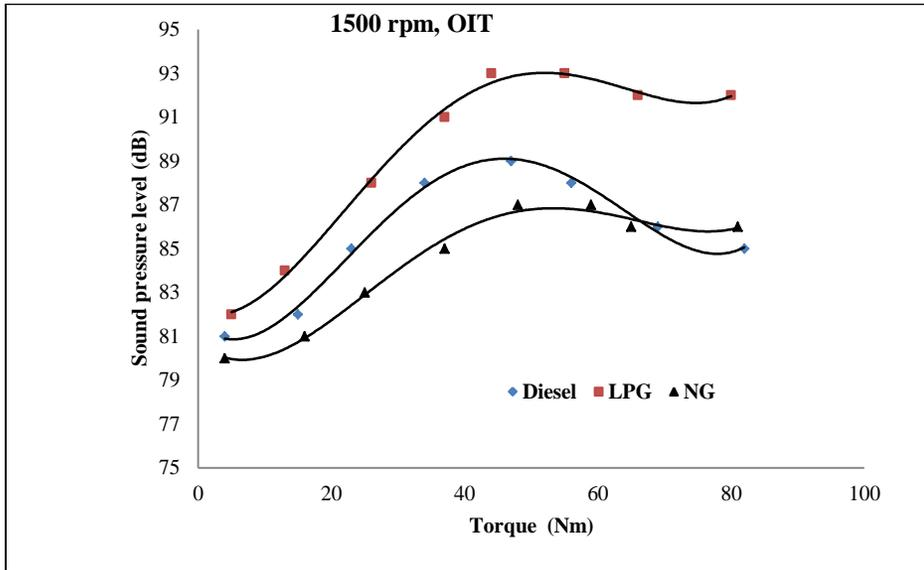
Fig. 5, The Effect of Load on Noise Levels for Variable Fuels at Constant Engine Speed and Optimum Injection Timing.
