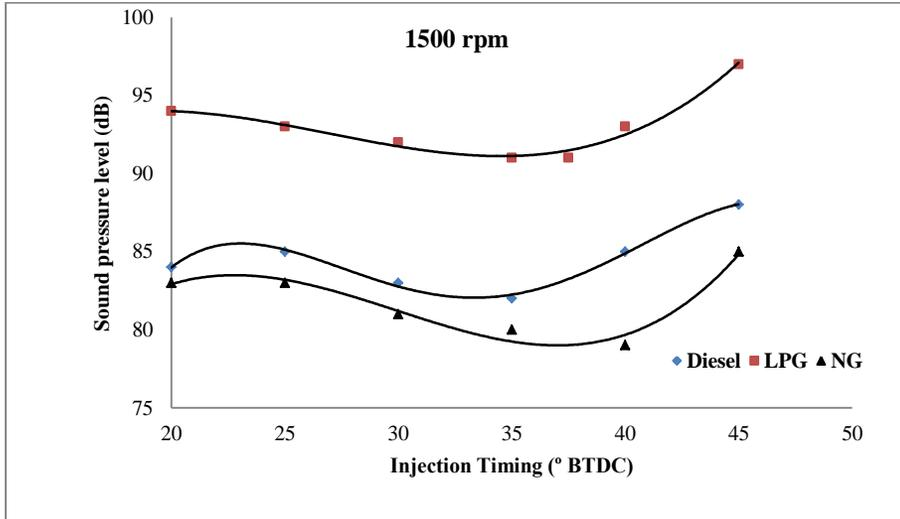
Fig. 10, The Effect Of Pilot Fuel Injection Timing On Noise Levels For Variable Fuels At Constant Engine Speed.
