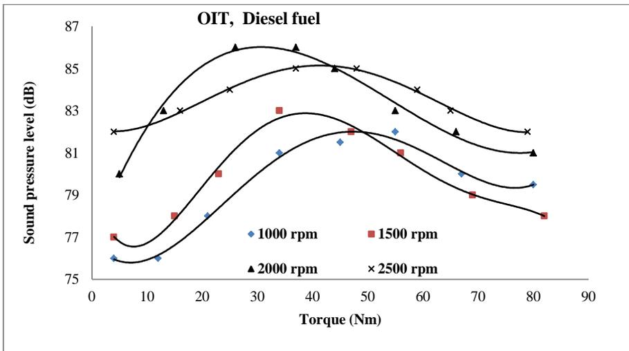
Fig. 6, The Effect of Load on Noise Levels for Diesel Fuel at Variable Engine Speed and Optimum Injection Timing.
