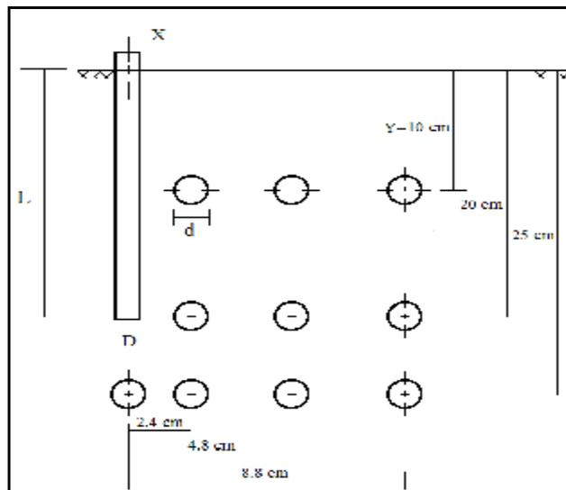
Figure (4): Problem geometry showing pile and cavity locations.
