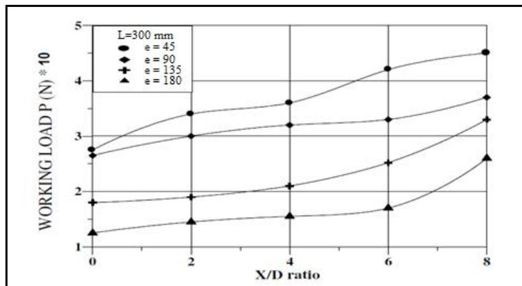
Figure (1): Variation of working load versus X/D at different load eccentricities (e) (group 5, three cavities, L= constant =300 mm) (after Al-Taie, 2004).
