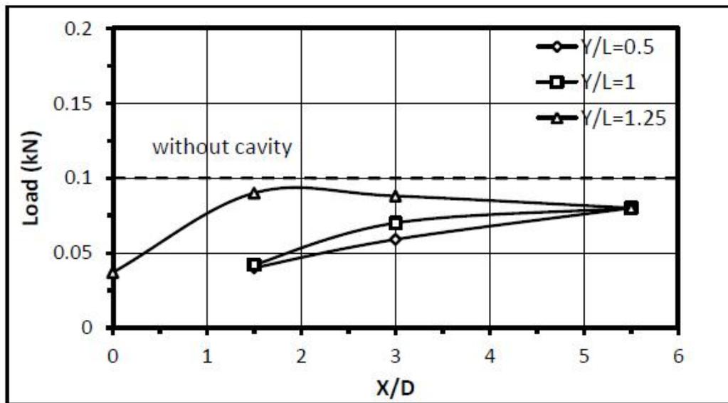
**Figure (7): Variation of single pile load versus cavity location of (X/D) at different depths of cavity with (d/D=1).**
