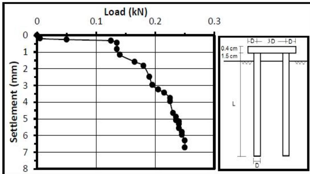
Figure (8): Load-Settlement curve of group piles (1x2) embedded in soil without cavity,  $L=20$  cm,  $D=1.6$  cm.
