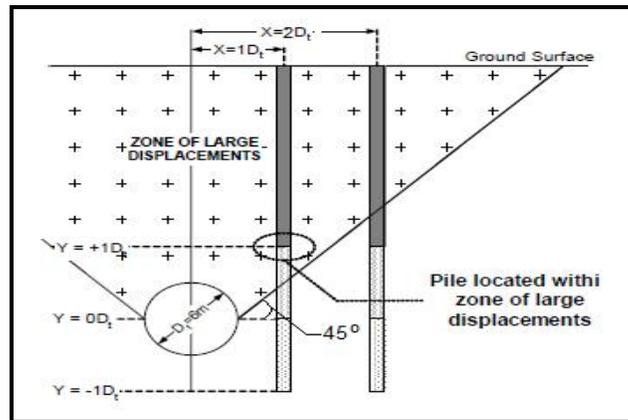
Figure (2): Location of pile tip relative to tunnel axis level and zone of large displacements (after Cheng et al., 2004).
