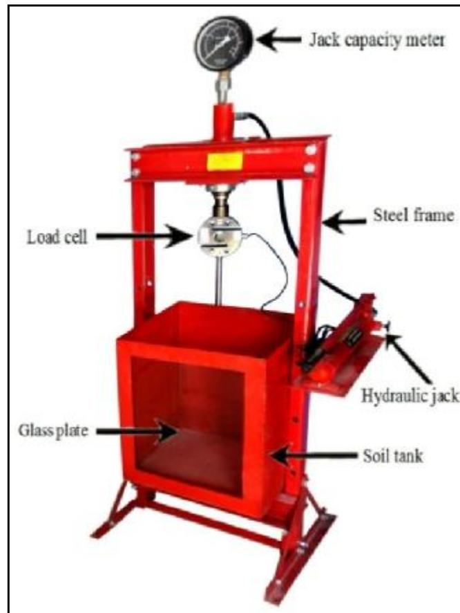
Plate (2): Testing setup.
