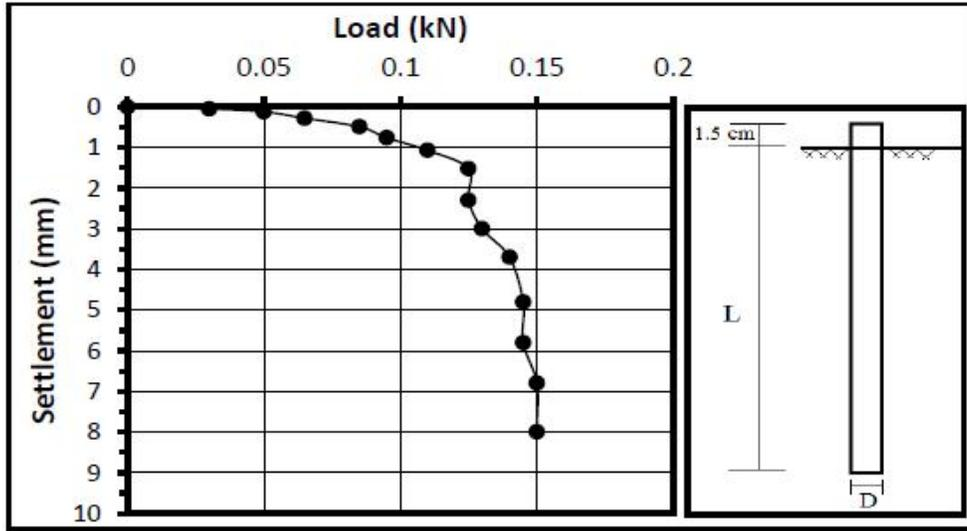
Figure (5): Load-settlement curve of single pile embedded in soil without cavity,  $L=20$  cm,  $D=1.6$  cm.
