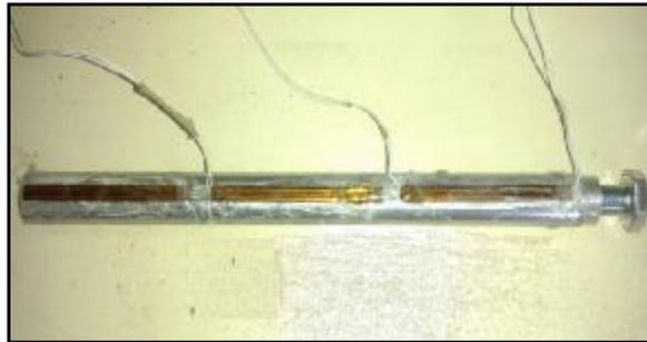
Plate (4): Attachment of strain gages to the pile.
