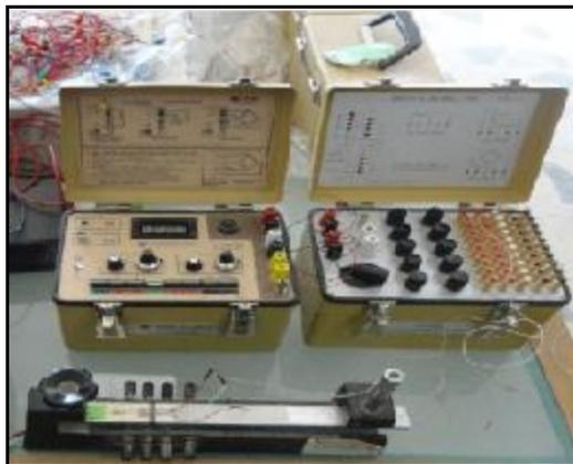
Plate (3): Calibration of the strain indicator.
