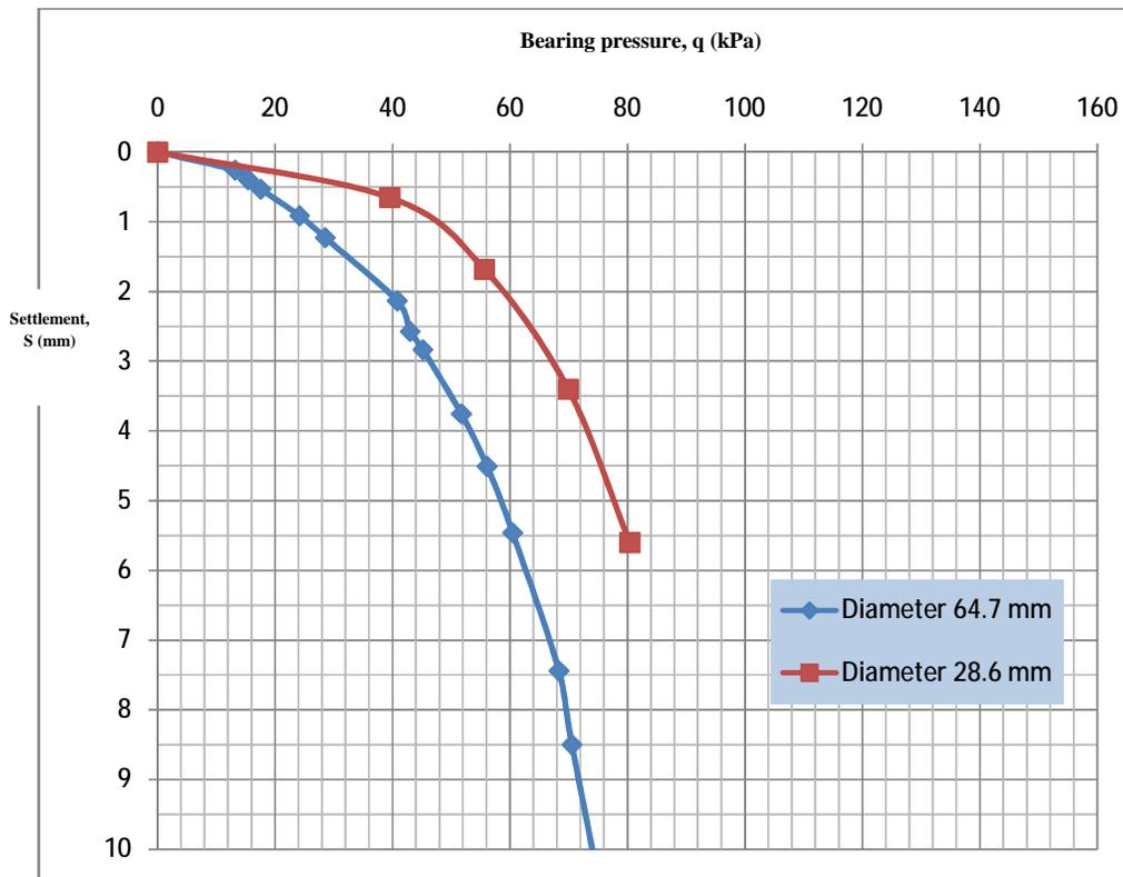
Figure (2): Bearing pressure versus settlement for untreated soil with different footing diameters.
