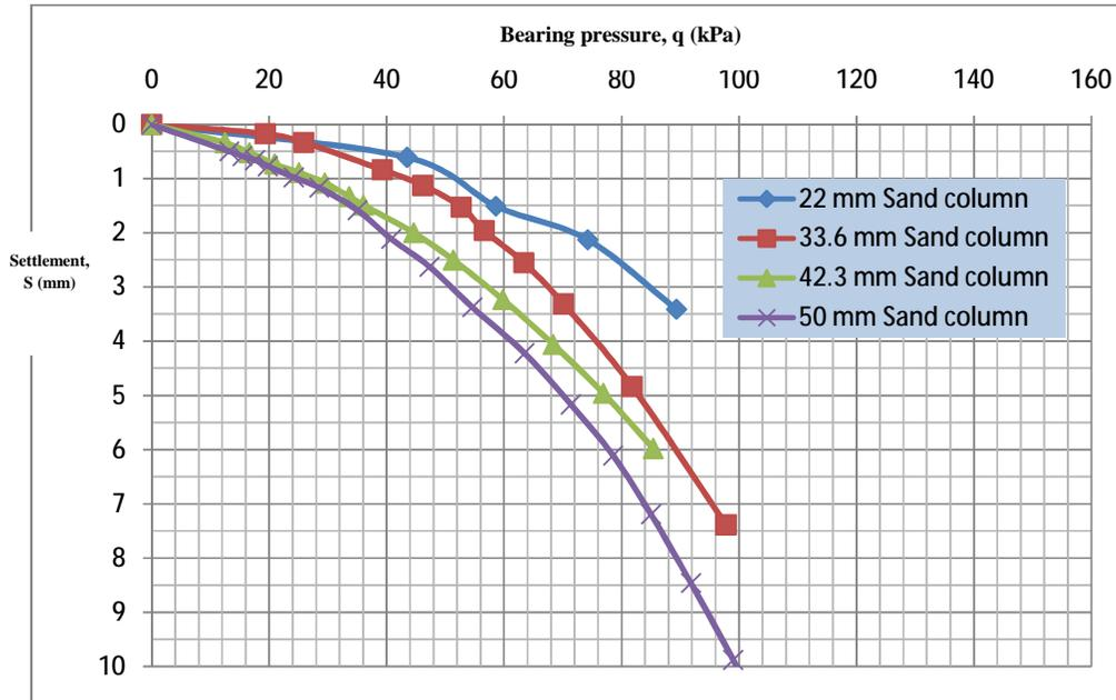
Figure (4): Bearing pressure versus settlement for soil treated with floating sand columns at loose relative density ( $\gamma=17 \text{ kN/m}^3$ ) with different diameters.
