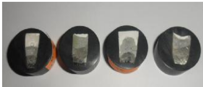
Figure (6): Sectioning and hot mounted of FGMs samples for metallographic observations.
