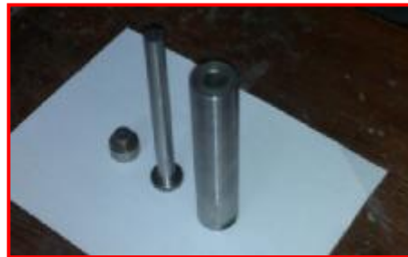
Figure (4): Cylindrical steel die with (15 mm) diameter.
