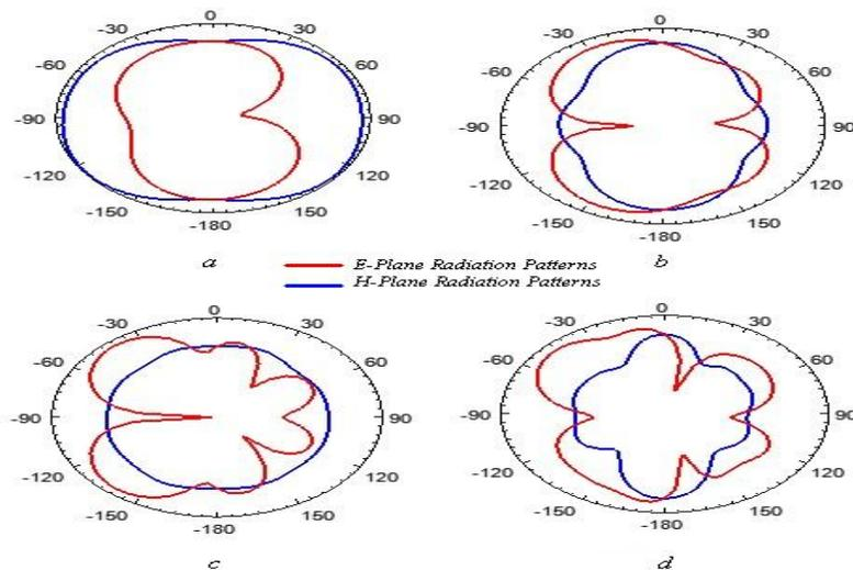
Figure (5). The simulated E-plane and H-plane radiation patterns of the proposed antenna at: (a). 0.90 GHz, (b). 3.0 GHz, (c). 3.8 GHz, and (d). 4.8 GHz.
