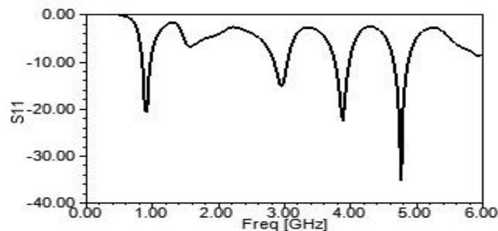
Figure (3). The simulated return loss response of the modeled antenna depicted in Figure(2).
