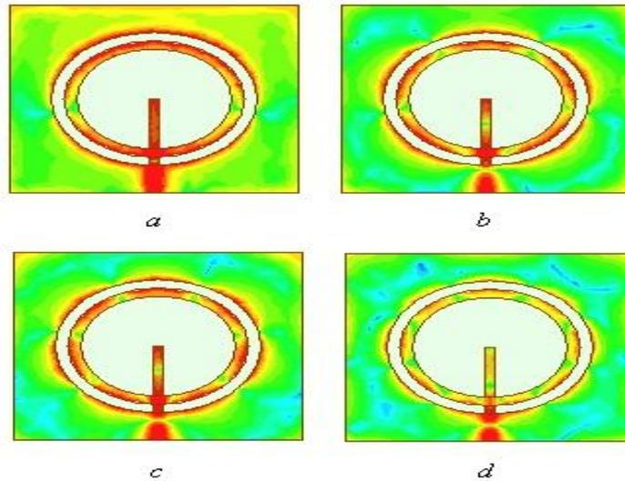
**Figure (6).** The simulated current distribution on the surface of the proposed antenna at: (a). 0.90 GHz, (b). 3.0 GHz, (c). 3.8 GHz, and (d). 4.8 GHz.
