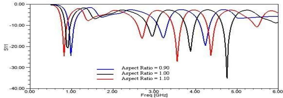
Figure (4). The simulated return loss responses of the proposed antenna for different values of antenna aspect ratio as a parameter: 0.90 (blue), 1.0 (black), 1.1 (red).
