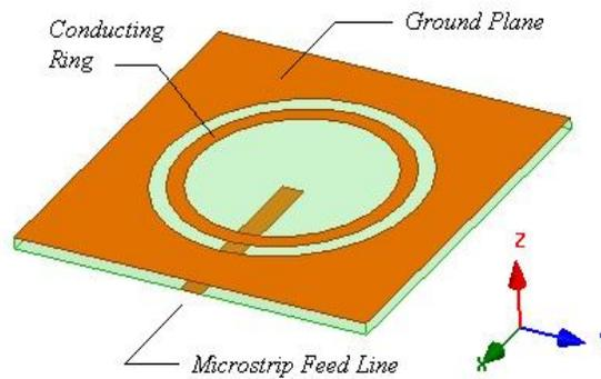
**Figure (2).** The proposed antenna layout with respect to the coordinate system.
