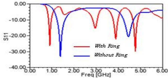
**Figure (7). The simulated return loss responses of the proposed antenna with and without the conducting ring.**
